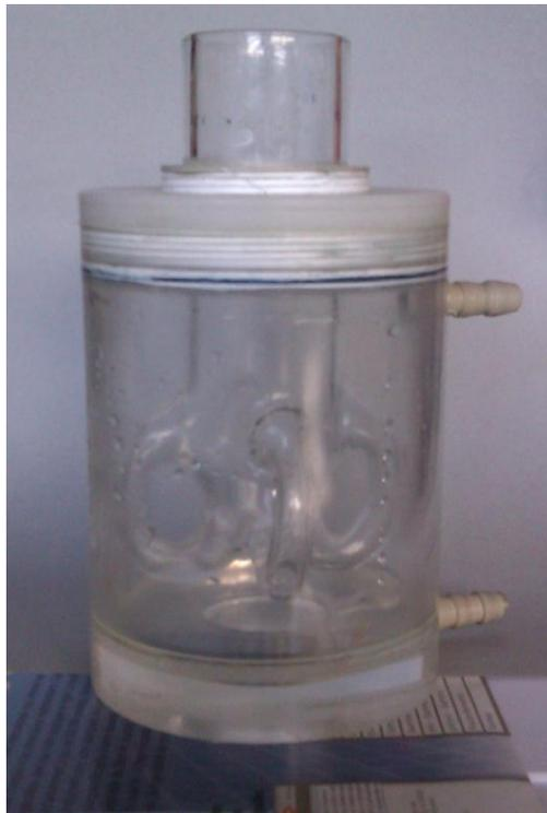
Fig. 1: Modified Rosett-type Reactor.
