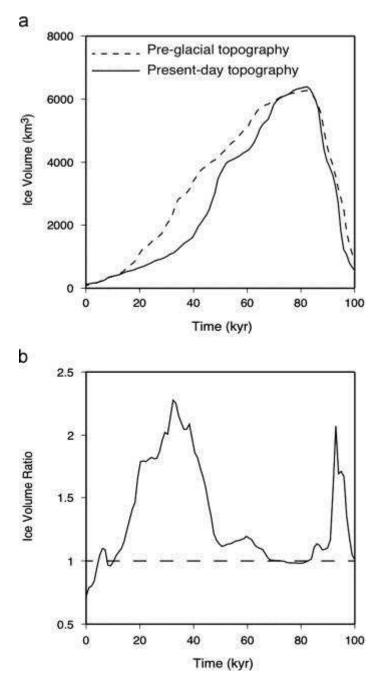
Fig. 3. : (a) Dashed and solid lines show the evolution of the ice volume through time on the pre-glacial and present-day topography, respectively (simulations A1 and A2, see text for details). (b) Ratio between pre-glacial and present-day ice volumes. The modeled ice volume on the pre-glacial topography surpass that of the present-day landscape by a factor of  $\sim 2$  during both the cooling and warming phases of the glacial/interglacial cycle.
