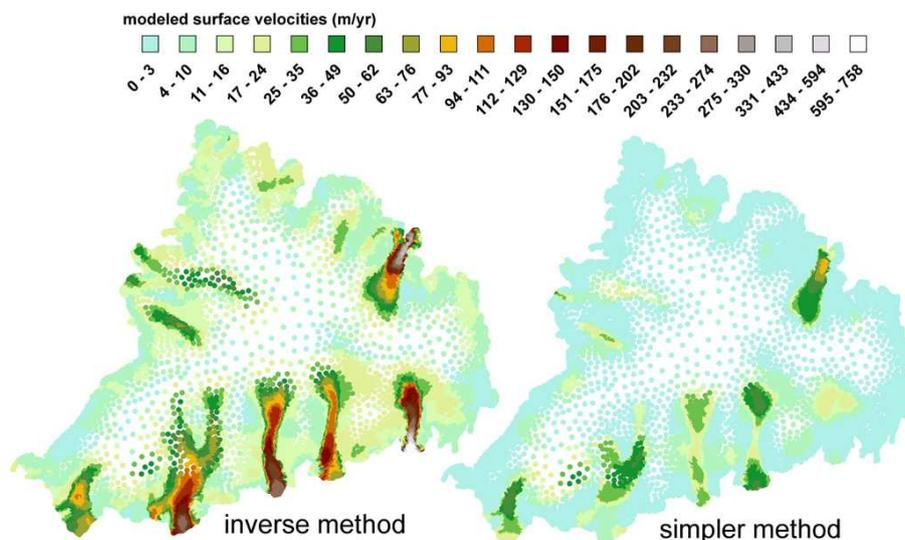
**Fig. 6.** Velocities obtained in a forward simulation by the model, on the left when using the basal distribution obtained with the inverse method, on the right by using a simpler approach: In each outlet glacier a different, but constant, sliding coefficient is used. The values here are in each outlet the mean values of the values obtained with the inverse method (Table 2).
