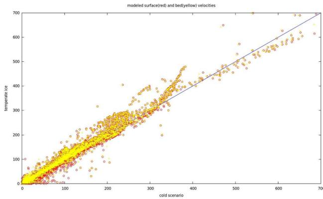
**Fig. 13.** Correlation between the modeled velocities for the two different temperature scenarios – for the surface velocities and respectively the basal velocities. Since the movement is dominated by the basal motion, there is hardly any difference between both velocity fields. All velocities are given in  $\text{m yr}^{-1}$ .
