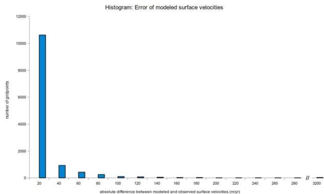
**Fig. 9.** Histogram of the difference between modeled and observed surface velocities. Note that the error on the measured surface velocities is  $7 \text{ m yr}^{-1}$  and that the last bin contains all entries with values higher than  $280 \text{ m yr}^{-1}$ .
