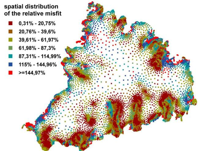
**Fig. 10.** Spatial distribution of the relative misfit between Neumann and Dirichlet velocities over the whole glacier surface. Comparison with Fig. 6 indicates that relative errors are similar in the fast-flow and slow-flow regime areas. The points with relative errors higher than 145% are highlighted in red to demonstrate that these are single points, mostly close to the margins.
