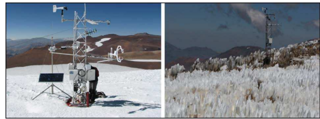
Fig. 8. Photographs taken on 23 January 2008 (mid-summer) at the level of the AWS for Guanaco Glacier (left) and Toro 1 Glacieret (right), see Fig. 3a and b for location. While the surface of Guanaco Glacier does not have penitents, Toro 1 Glacieret is completely covered by penitents of snow (in the foreground) and of ice (in the vicinity of the AWS).
