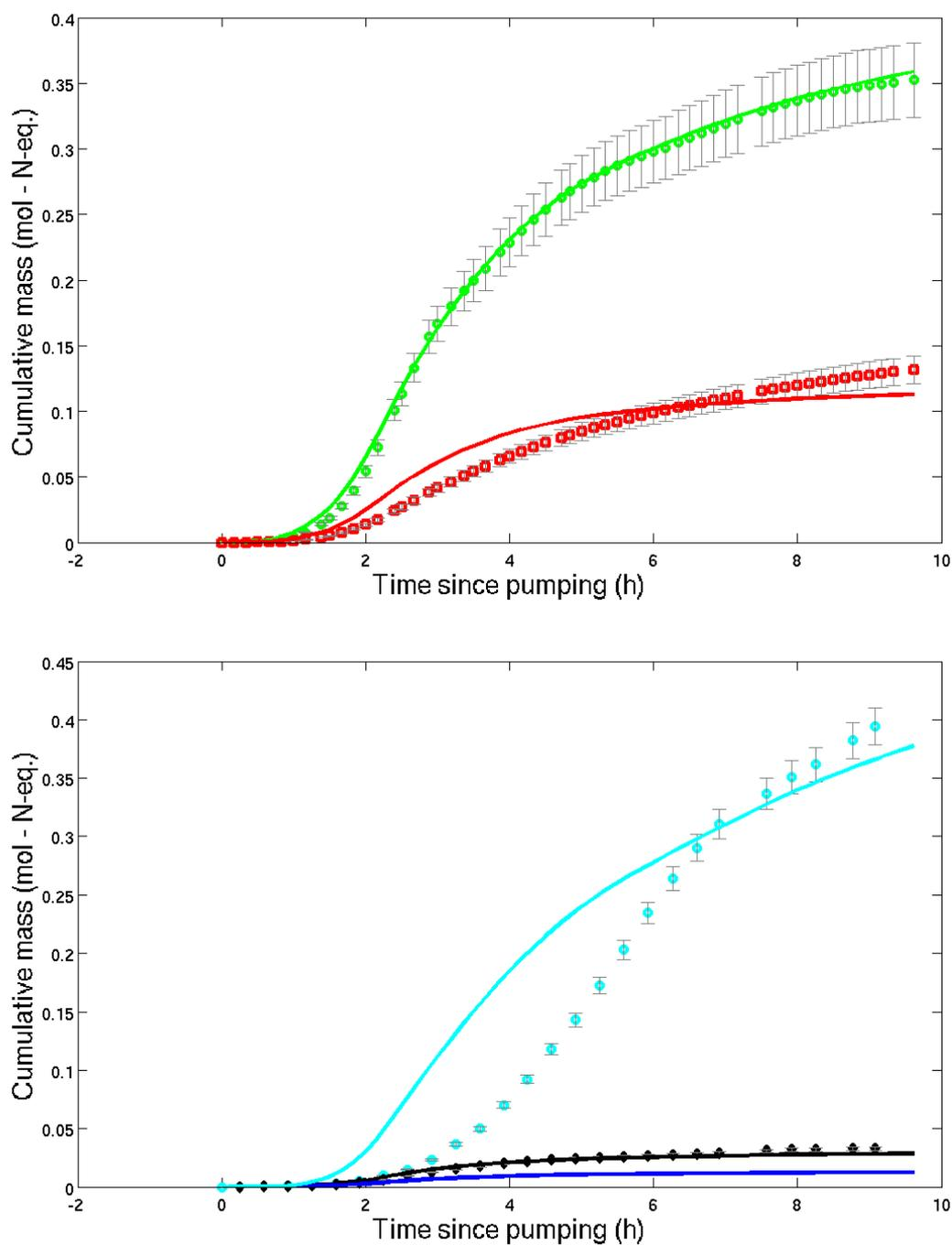
Fig. 5: Cumulative mass of the total reduced  $\text{NO}_3^-$  (a-green); produced  $\text{NO}_2^-$  (a-red); produced  $\text{N}_2\text{O}$  (b-black) and  $\text{N}_2$  (b-cyan). Curves represent model results for each compound. The blue line (b) represents the estimated  $\text{NO}$  mass production. The dashed line represents theoretical  $\text{N}_2$  production. Error bars represent the analytical error..
