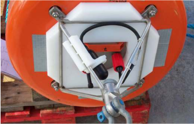
Figure 4 The hydrophone instrument is housed inside the buoy just before deployment. The sensor is attached to the buoy frame and plugged into the instrument.
