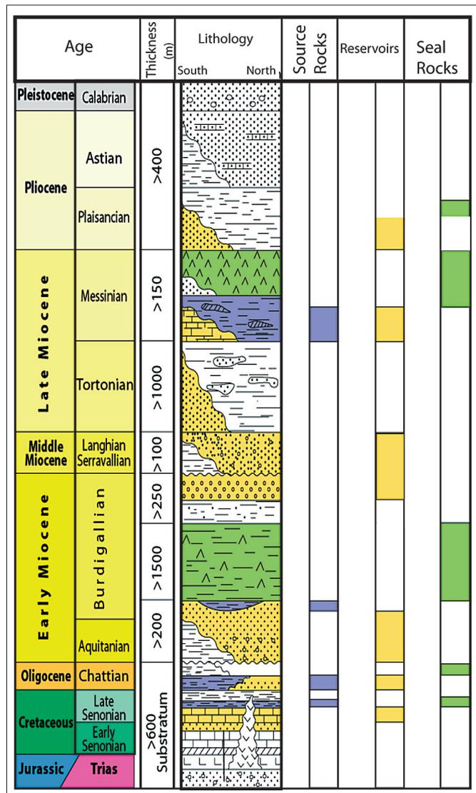
Figure 5. Generalized stratigraphic chart of the onshore Cheliff Basin and its petroleum systems as an exploration analog for the offshore area.
