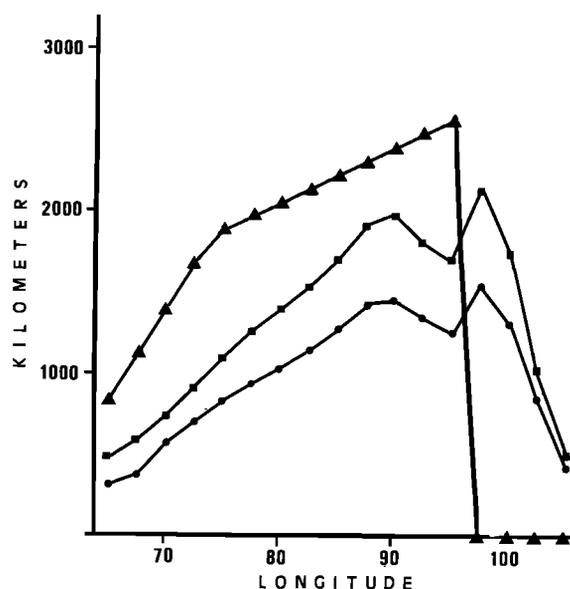
Fig. 5. The equivalent linear shortening as in Figure 4 is shown here corrected for erosion and for the 45 Ma topographic base level. It is compared to the expected linear shortening from kinematics (upper curve with triangles). Two cases are shown for two different topographic base levels at 45 Ma: the 0 m case (curve with squares) and the 500 m one (curve with small circles). See text for discussion.
