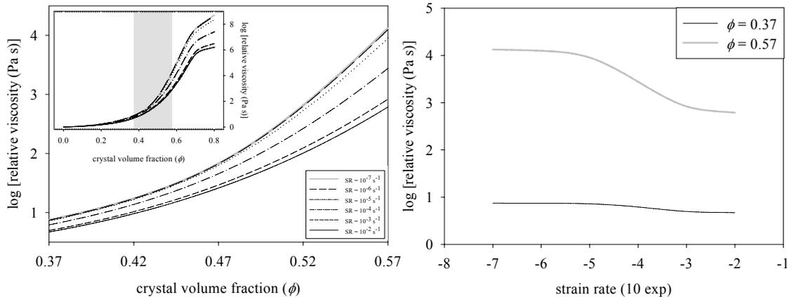
**Fig. 4.** (a) Relative viscosity as a function of crystal volume fraction at different strain-rates; (b) relative viscosity as a function of strain-rate for two crystal volume fractions of 0.37 and 0.57, adopted for fire-fountain and Strombolian phases of the Etna 2000 activity, respectively. Calculations made with the model in Costa et al. (2009).
