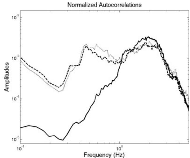
**Figure 2.** Normalized average autocorrelations of horizontal and vertical motion at the Texcoco site. Vertical and horizontal (NS and EW) motions are represented with continuous and dashed lines, respectively. Duration of windows is 40 s. For details see the Supplementary Information.
