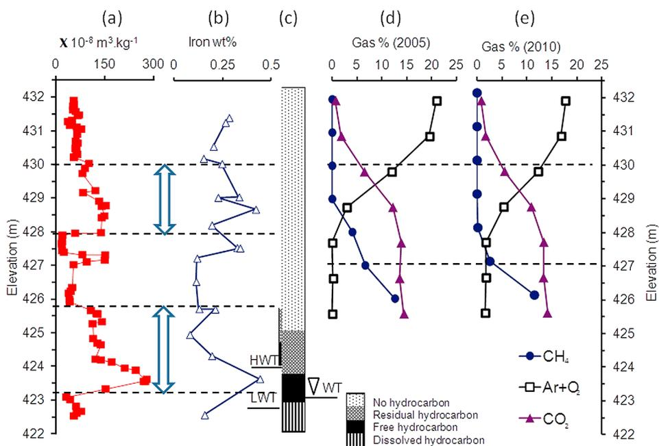
**Figure 2.** (a) Magnetic susceptibility, (b) iron wt %, (c) hydrocarbon distribution within core, gas concentrations in (d) 2005, and (e) 2010 along the contaminated core (C 1010). HWT: Highest water level, LWT: Lowest water level and WT: Water Table during the time of measurements. Elevation above mean sea level (amsl). The gas data are from location 534 located 10 m from C1010.
