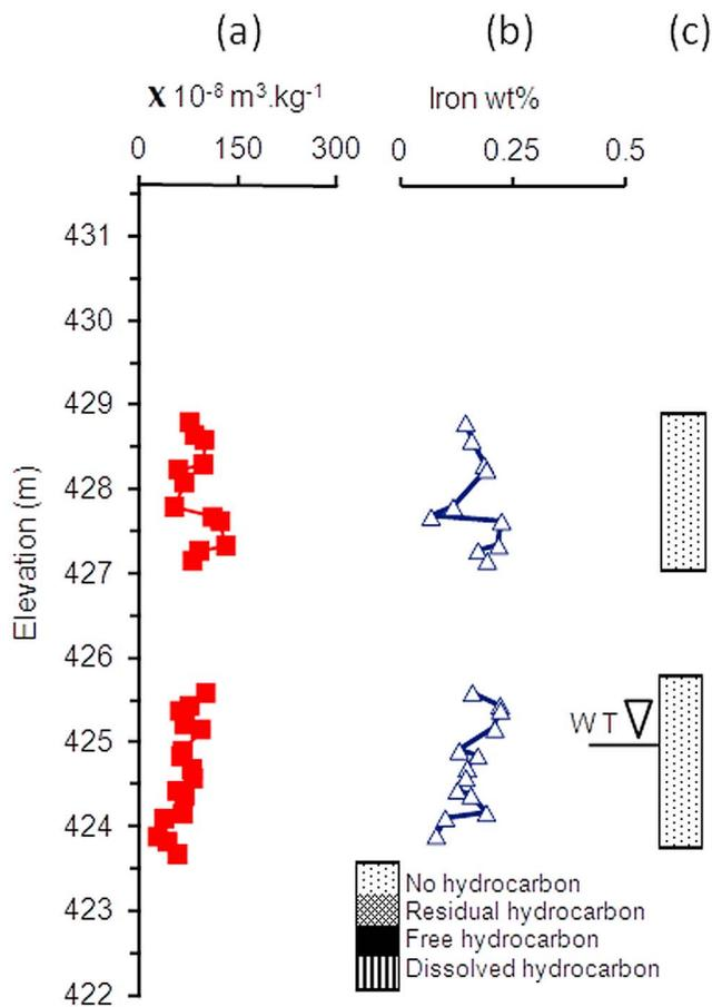
**Figure 3.** (a) Magnetic susceptibility, (b) iron wt %, and (c) hydrocarbon distribution in two 2-m zones along the uncontaminated borehole (C 1006). WT: Water Table during the time of measurements. Elevation above mean sea level (amsl).
