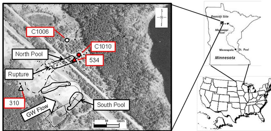
**Figure 1.** Study area showing the location of core samples (circles) and gas data (triangles) at contaminated (closed symbols) and uncontaminated (opened symbols) boreholes. 310 and 534 are vadose zone gas sampling boreholes.
