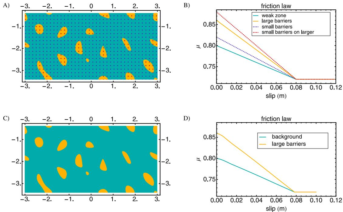
**Figure 9.** A model with two-scale heterogeneity (a) values of  $\mu_s$  on the fault, non regular at large scale, regular at small scale, and (b) corresponding linear friction laws. (c and d) Small-scale heterogeneity is removed and replaced by the effective friction law. Slip evolution of these two models can be seen in Figure 10.
