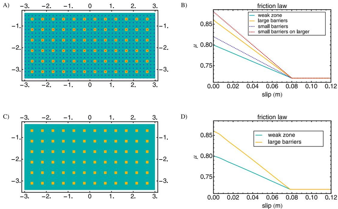
**Figure 7.** A model with two-scale heterogeneity (a) values of  $\mu_s$  on the fault and (b) corresponding linear friction laws. (c and d) The small-scale heterogeneity is removed and replaced by the effective friction law. Slip evolution on these two models can be seen in Figure 8.
