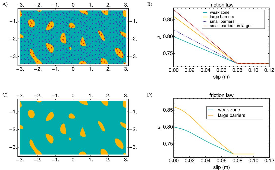
**Figure 11.** A model with two-scale uneven heterogeneities (a) values of  $\mu_s$  on the fault, and (b) corresponding linear friction laws. (c and d) Small-scale heterogeneity is removed and replaced by the effective friction law. Slip evolution on these two models can be seen Figure 12.
