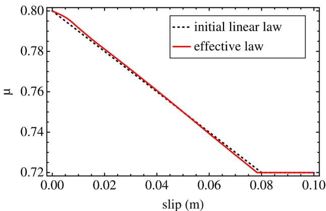
**Figure 4.** The effective friction law (plain curve) constructed to account for small-scale heterogeneities of the heterogeneous model. Compared to initial linear slip-weakening friction-law (dashed curve), the initial slope is smaller (slower initiation), until breaking of the barrier leads to a kink and a steeper curve corresponding to the acceleration of the initiation process.
