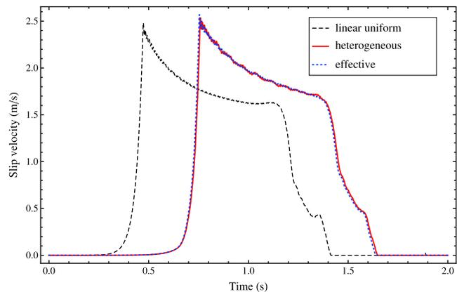
**Figure 5.** Slip velocity on the center of the fault for the uniform linear, heterogeneous and effective model. The effective friction law permits to reproduce the delay of initiation due to heterogeneity and the shape of the velocity history after the weakening phase with very good agreement.
