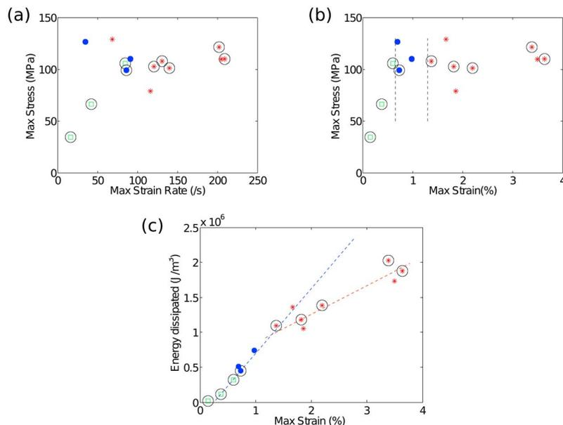
**Figure 3.** Phase diagrams of the macroscopic damage patterns. (a) Maximum strain rate vs. maximum stress. (b) Maximum strain vs. maximum stress. (c) Dissipated energy vs. maximum stress. Green squares, blue circles, and red asterisks indicate, respectively, apparently intact, split, and pulverized samples. Jacketed samples are indicated with a circle surrounding the damage symbol.
