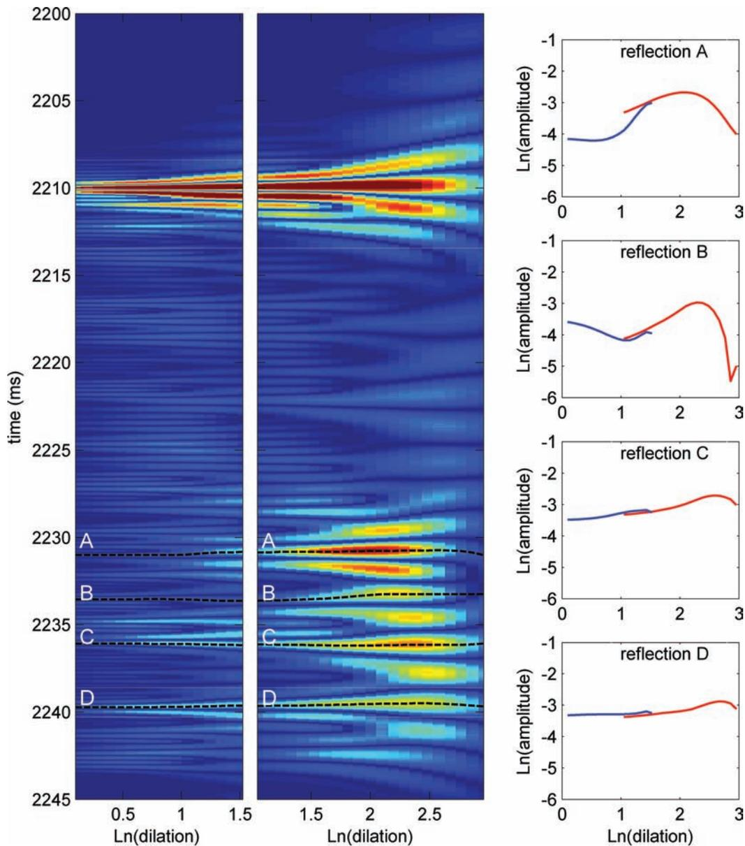
**Figure 8.** (a and b) Modulus of the synthetic wavelet responses (WR) including band-limited frequency of the seismic source in the VHR (580–2200 Hz) and HR (220–1050 Hz) domains, respectively, and selected ridge functions. (c, d, e and f) Compensated ridge functions, in the VHR (blue) and HR (red) domains.
