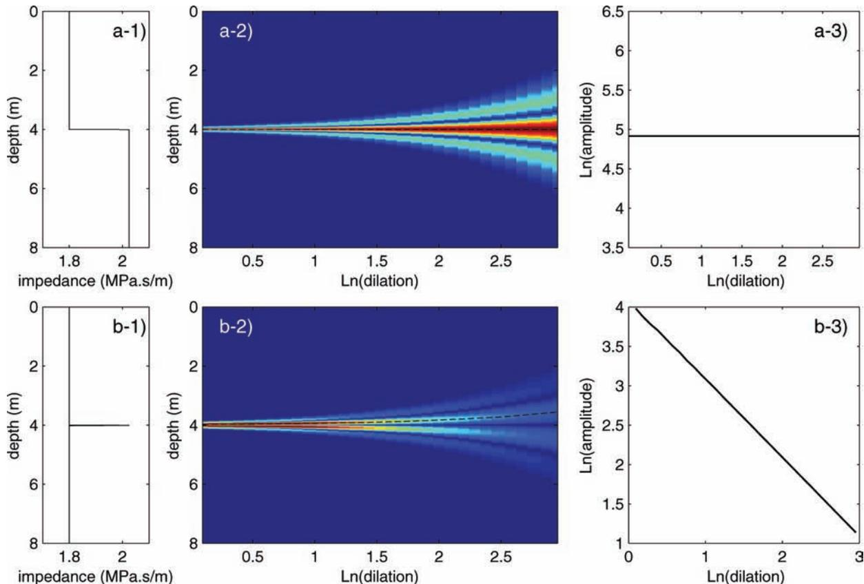
**Figure A1.** Top panels (left- to right-hand side): Heaviside step function, CWT modulus and ridge function. Bottom panels (left- to right-hand side): Dirac impulse function, CWT modulus and ridge function.
