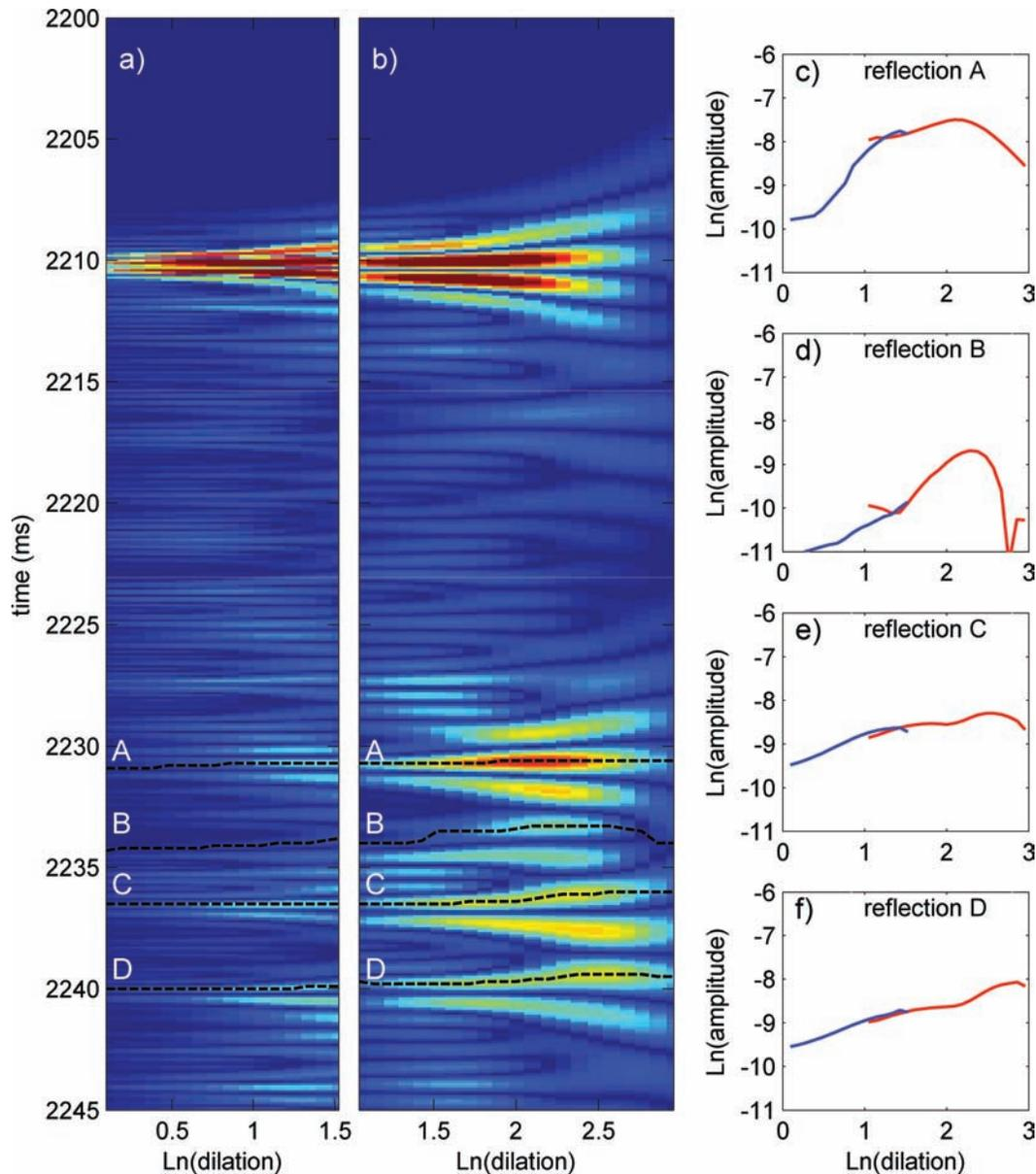
**Figure 7.** (a and b) Modulus of the wavelet transforms (WT) of the deep-towed seismic trace in the VHR (580–2200 Hz) and HR (220–1050 Hz) domains, respectively, and selected ridge functions in dashed lines. (c, d, e and f) Compensated ridge functions, in the VHR (blue) and HR (red) domains.
