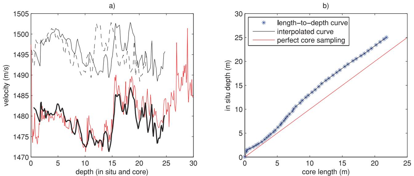
**Figure 3.** (a).  $P$ -wave velocity profiles: PENFELD *in situ* measurements (red), laboratory core measurements (dashed) + length-to-depth law correction (black) + environmental corrections (bold). (b) Length-to-depth relationship provided by the coring monitoring.
