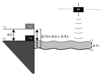
**Fig. 1.** Relationships between the relative sea level change at tide gauges  $\Delta T.G.$ , absolute sea level change  $\Delta S.L.$  given by satellite altimetry and net ground motion  $\Delta G.$  Alt: altimeters; T.G.: tide gauge. t1 and t2 are two different times or record.
