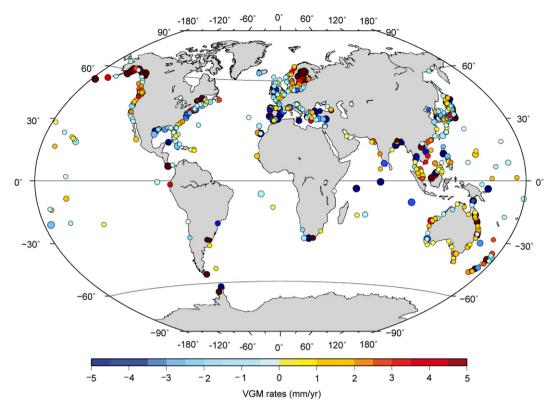
Fig. 2. Vertical ground motion (VGM) rates calculated in our study based on the difference between the records from satellite altimetry and tide gauge records. The colour scale is bounded to  $\pm 5$  mm/yr but actual values range between -53 and 35 mm/yr. The point size varies according to the quality of the fit ( $R^2$  ranging from 0 to 0.95).
