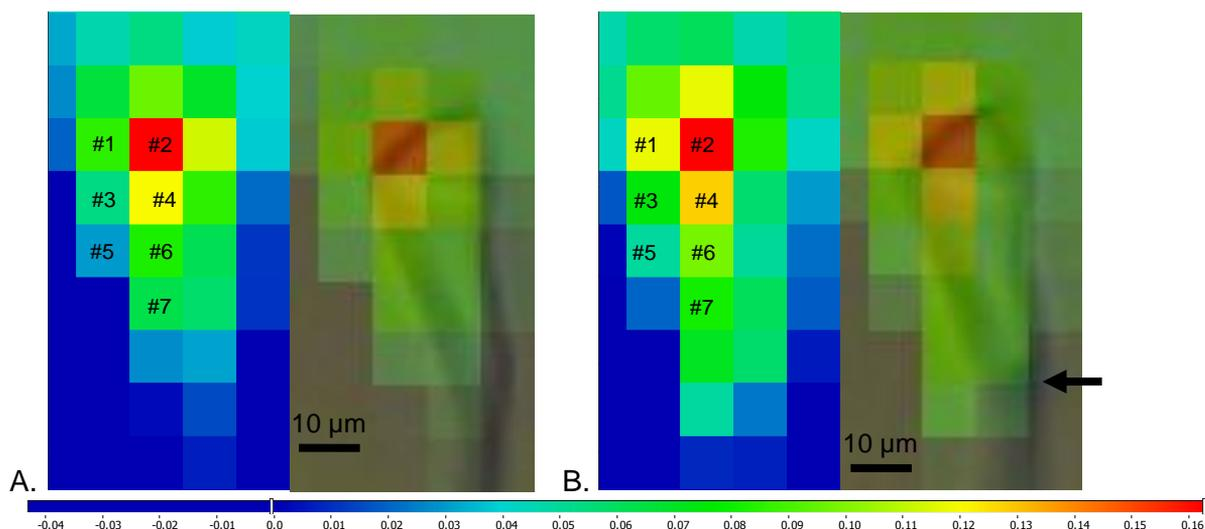
Figure 3. IR map of the sampled inclusion in the sample 1, before (3A) and after (3B) nucleation. Each square scales the beam size ( $8 \times 8 \mu\text{m}$ ) over each recorded spectrum, and the colour relates to the absorbance scale, taken at the main peak of the OH-stretching band:  $3640 \text{ cm}^{-1}$ .
