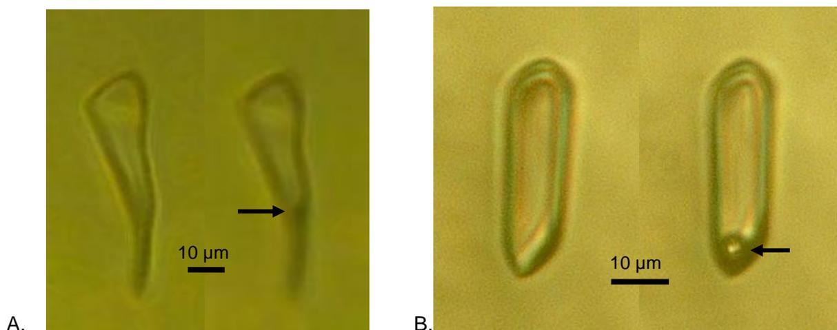
Figure 2. Photographs of the sampled fluid inclusions (A. sample 1; B. sample 2). On the left of each sub-figure, the monophasic inclusions contain the superheated liquid. To the right, the same inclusions after nucleation (biphasic mixture), the arrows point to the visible bubble.
