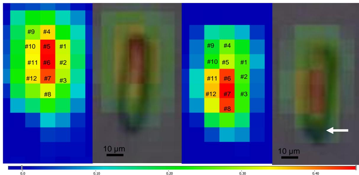
Figure 4. IR map of the sampled inclusion in the sample 2, before (two left photos) and after (two right photos) nucleation. Each square scales the beam size ( $8 \times 8 \mu\text{m}$ ) over the recorded spectrum, and the colour relates to the absorbance scale, taken at the main peak of the OH-stretching band:  $3570 \text{ cm}^{-1}$ .
