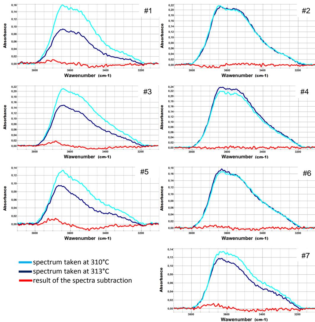
Figure 5. Baseline-corrected spectra of metastable superheated (at 313°C) and stable water (at 310°C) in the sample 1. The numbers relate to the location on the map (see Fig. 3).
