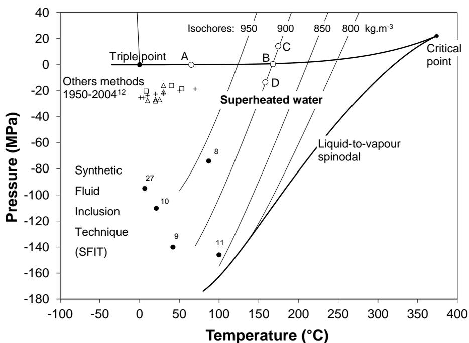
Figure 1. Phase diagram of water (IAPWS-95 equation of state<sup>13</sup>), extended to the superheated water domain. Experimental measurements of the extreme tensile strength are reported. The classic microthermometric path (see text) is reported from the ambient conditions (A) to the homogenization temperature (Th, B), possibly up to overheating conditions (C), and cooled after down to the nucleation temperature (Tn, D) (see text).
