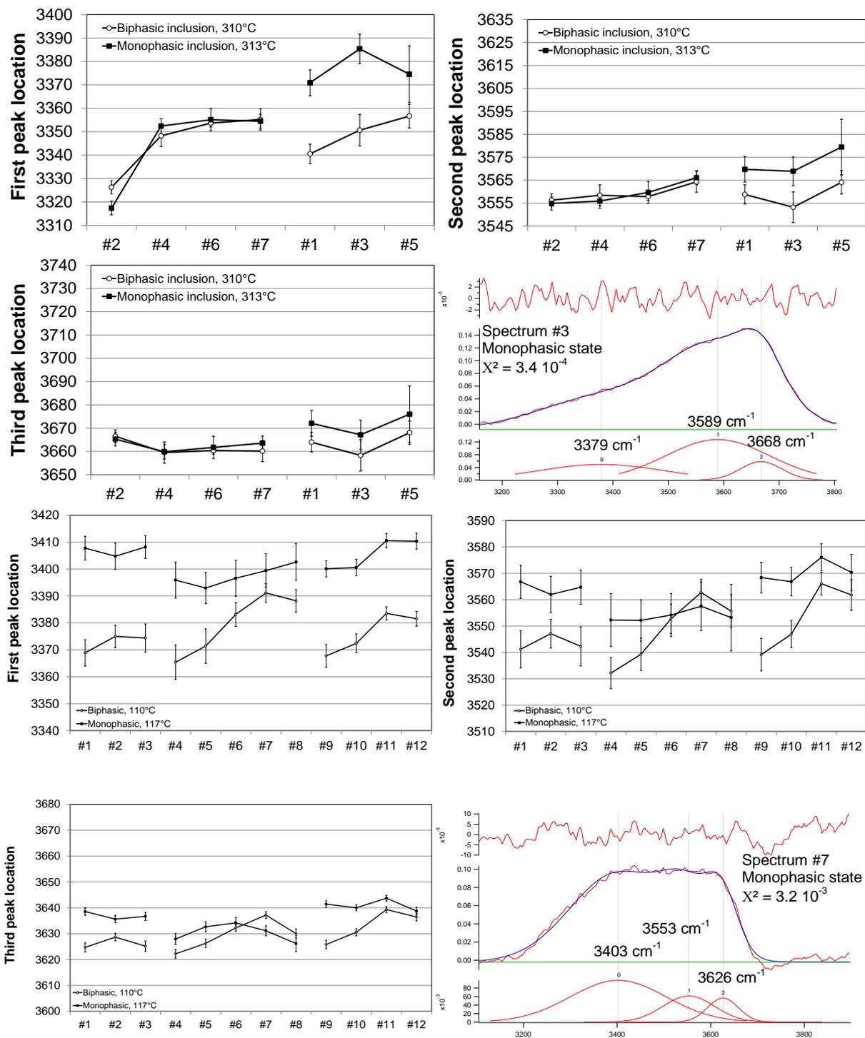
Figure 7. Decomposition of the OH-stretching band into three sub-bands (see text), for the samples 1 (four upper graphs), and 2 (four lower graphs). All the ordinates axis are plotted over the same  $90 \text{ cm}^{-1}$  interval.
