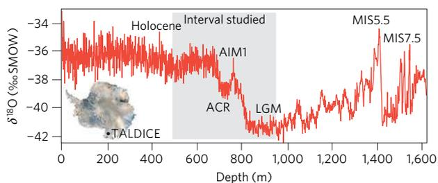
**Figure 1 | The TALDICE stable isotope profile ( $\delta^{18}\text{O}$ ) versus depth.** The interval studied (8–25 kyr BP) is marked with grey shading. MIS 5.5, 7.5, LGM, AIM1 and ACR are indicated. The satellite image of Antarctica shows the location of the TALDICE ice core.
