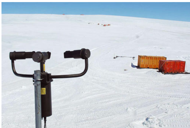
Fig. 12. Biral VPF730 in Antarctica.
