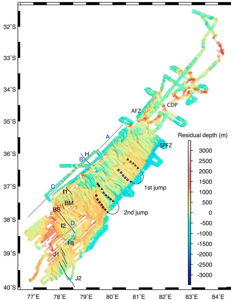
**Figure 4.** Residual depths computed from the multibeam bathymetry and the removal of a subsidence trend with the square root of age. Depths around “zero” correspond to normal depths for the considered age. Depths were not corrected for the effect of sediment loading, since sediment thickness was found to be relatively uniform and relatively thin over most of the area. Thin black lines, black arrows and magenta, red symbols and labels as for Figures 1 and 2.
