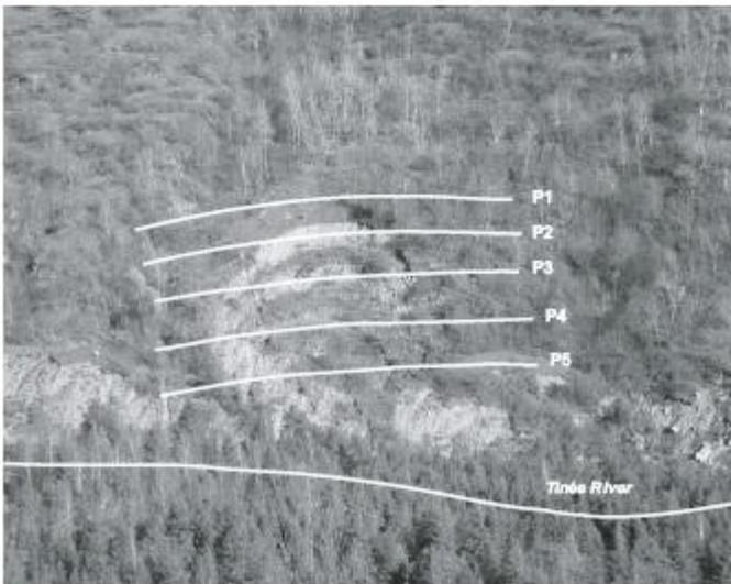
Fig. 4 Location of the five electrical profiles on the Clapiere landslide.
