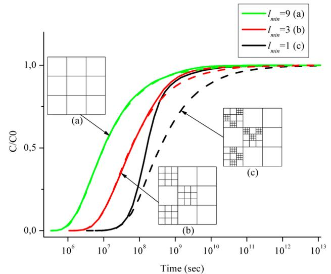
**Figure 4.** Breakthrough curves for hierarchical fracture networks with different fracture resolutions. The length of the smallest fracture ranges from 1 m to 9 m (from the green curves to the black curves) with a domain size of 27 m. Dashed lines show results assuming infinite matrix, whereas solid lines show results by accounting for the effect of the neighboring fractures.
