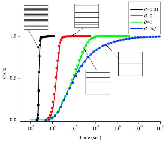
**Figure 3.** Breakthrough curves for a set of parallel fractures (black, red, and green curves) with different fracture spacings ( $B$ ) and for a single fracture (blue curve). Solid lines and squares represent analytical solution and numerical results, respectively.
