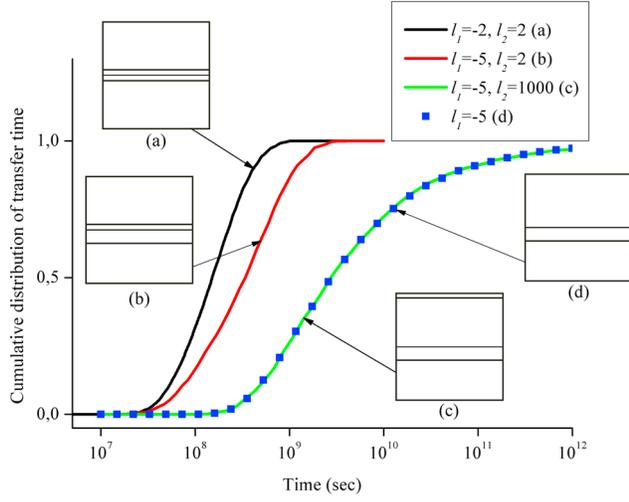
**Figure 2.** Cumulative distribution of the transfer time to nearby fractures. Particles transfer from position  $x = 0$  to positions  $x = l_1$  and  $x = l_2$ . Solid lines and dots represent results obtained with Feller and FPTD formulations, respectively. The local diffusion coefficient is equal to  $10^{-8}$  m<sup>2</sup>/s, and the fracture positions are expressed in meters.
