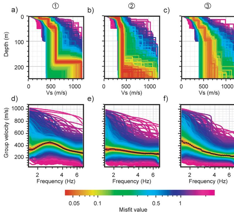
**Figure 10.** (a–c)  $V_s$  profiles resulting from the inversion of the local dispersion curves of cells 1–3 in Figure 8 with the parameter space described in Table 2. (d–f) Colors show the corresponding dispersion curves; black shows the inverted dispersion curves measured by tomography.
