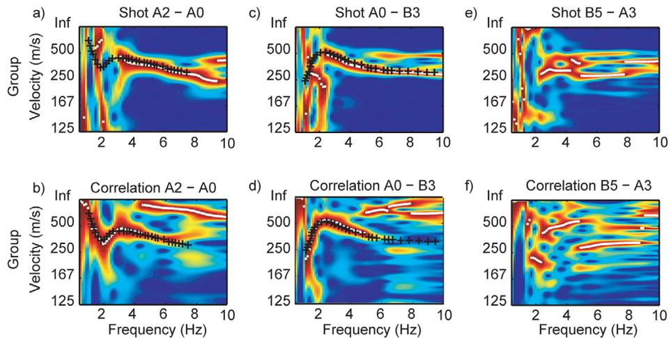
**Figure 7.** Rayleigh wave group velocity dispersion images computed on (a, c, and e) shots and (b, d, and f) cross-correlated signals for propagation from A2–A0 (Figures 7a and 7b), A0–B3 (Figures 7c and 7d), and B5–A3 (Figures 7e and 7f). Black crosses correspond to the picked velocity values for paths A2–A0 and A0–B3. No Rayleigh dispersion curve can be identified on the B5–A3 images, where the energy is completely split, certainly owing to the medium complexity.
