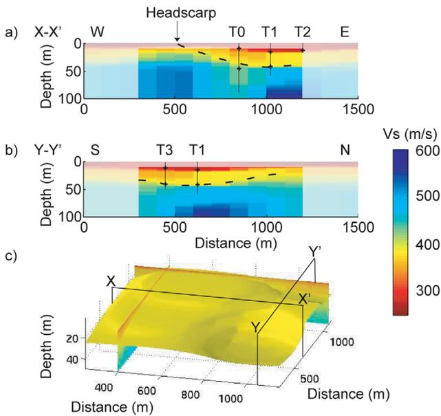
**Figure 12.** Comparison with previous investigations. Sections (a)  $X-X'$  and (b)  $Y-Y'$  down to 100 m. Their locations are given in Figure 12c. Crosses are depths of slip surfaces found in boreholes T0–T3; arrow shows the location of landslide headscarp; and dashed line is the interpreted deepest limit of the landslide. (c) Three-dimensional view of the 380 m/s isosurface, which approximately corresponds to the landslide deepest sliding surface.
