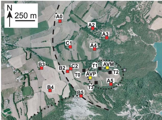
**Figure 2.** Acquisition layout on the landslide with 11 stations of the HRI network (red squares) and two permanent stations AVP and AVM (yellow squares). Dashed line is the outer limit of the Avignonet landslide. Dotted line is the limit of the Harmalière landslide. Dashed ellipse is the most active part of the landslide. Black squares show the locations of the four boreholes T0–T3 mentioned in section 6. Gray star shows the location of the outcrop of the glaciofluvial deposits.
