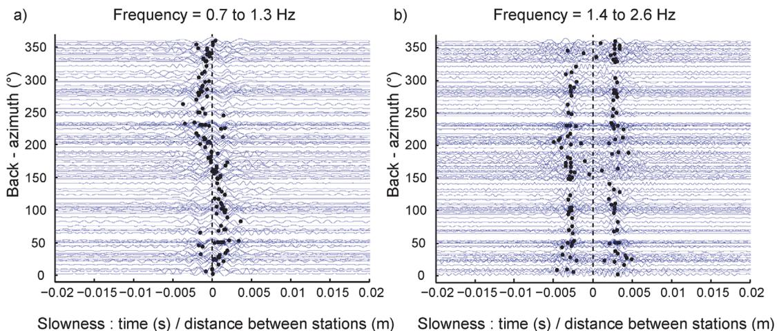
**Figure 6.** Cross correlations scaled by their interstation distance plotted versus the back-azimuth of the station pair and filtered between (a) 0.7 and 1.3 Hz and (b) 1.4 and 2.6 Hz. Black points correspond to the maximum of the envelope of the signals.
