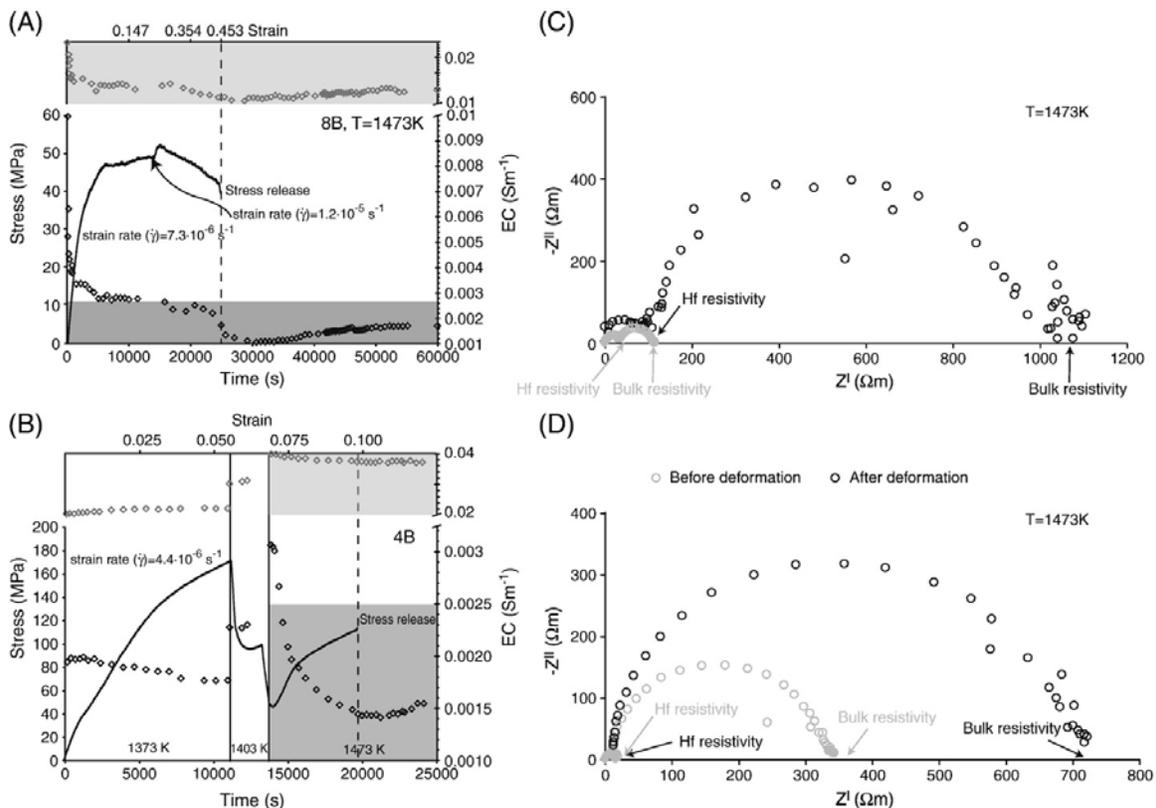
**Figure 5:** Variation of stress and EC during deformation of sample 8B (A) and 4B (B) with increasing deformation. The black lines give the variation of stress with increasing time and strain, the grey symbols show the EC associated to the HF conduction
