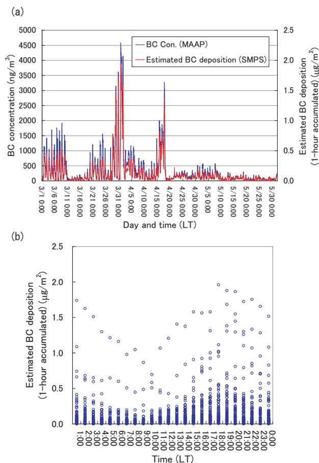
**Fig. 3.** (a) One-hour mean eqBCC from MAAP data (Bonasoni et al., 2008) and estimated hourly total BCD flux (right side scale) as multiplying dry deposition amount from SMPS data by 0.087 during March–May in 2006; (b) Composite of the estimated hourly total BCD flux during March–May in 2006.
