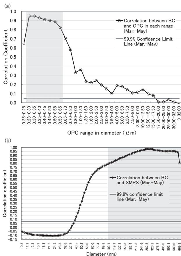
**Fig. 2.** Correlation coefficients (black solid line with circle) for March–May in time series data between atmospheric eqBCC and (a) particle counts in each size (as measured by OPC); (b) (as measured by SMPS). The bold line in gray denotes 99.9% confidence limit lines. The shade size ranges correspond to the correlation coefficient of more than 0.8.
