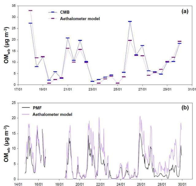
**Fig. 10.** Inter-comparisons of the time series of  $OM_{wb}$  concentrations calculated by the different source apportionment models. (a) Outputs of the CMB and Aethalometer models (12h-averaged data, from 17 January 2009, 18:00 to 30 January 2009, 06:00). (b) Outputs of the AMS-PMF and Aethalometer models (15 min-averaged data, from 14 January 2009, 16:00 to 29 January 2009, 23:30).
