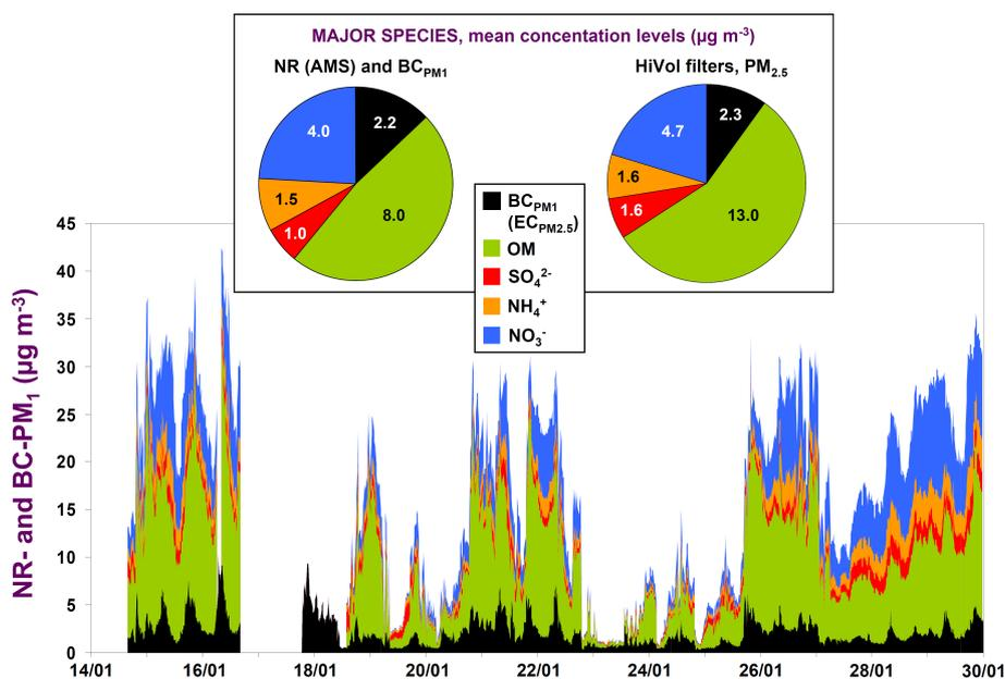
**Fig. 1.** Time series and mean concentration levels of the main components of the fine aerosol fraction during the period of study. Due to technical issues, AMS measurements are not available from 16/01 to 18/01. Mean  $PM_{2.5}$  concentrations and  $BC_{PM1}$  were calculated during the same periods than AMS measurements (upper panel).
