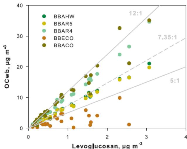
**Fig. 3.** Biomass burning organic carbon ( $\text{OC}_{\text{wb}}$ ) estimated using CMB modeling with the five selected biomass burning profiles as a function of levoglucosan. The dotted grey line represents the  $\text{OC}_{\text{wb}}$ -to-levoglucosan ratio recommended by Puxbaum et al. (2007) for European background environments, while grey lines as used here as indicators.
