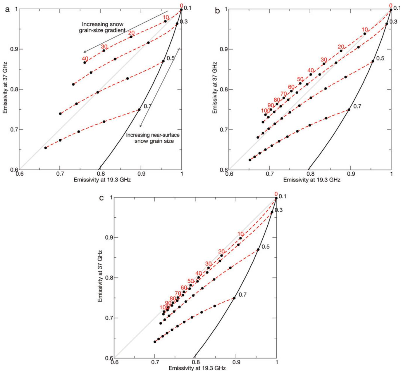
**Fig. 6.** Modeled emissivities of homogeneous snowpacks (black curve) and of snowpacks with a linear increase of (a) snow grain radius ( $n = 1$ ), (b) grain surface area ( $n = 2$ ) and (c) grain volume ( $n = 3$ ). The dashed red curves represent an increase in the grain-size gradient for a given near-surface snow grain size (Equation (2)). Annotated values along the dashed curve are  $Q_n$  ( $\text{m}^2 \text{m}^{-1}$ ) and along the homogeneous curve are the near-surface grain size (mm).
