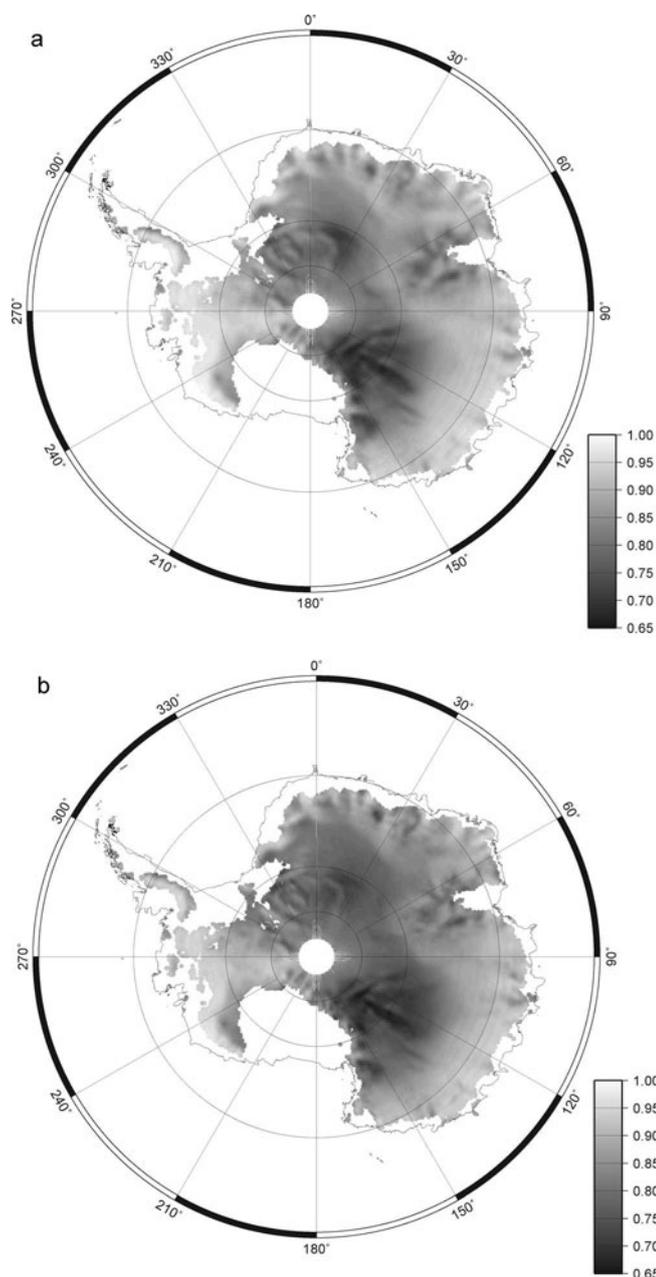
**Fig. 1** Maps of observed emissivities at vertical polarization (a) 19.3 GHz and (b) 37 GHz computed using Equation (1). Regions where melt occurred are masked (in white). No data are available south of 87.8°.
