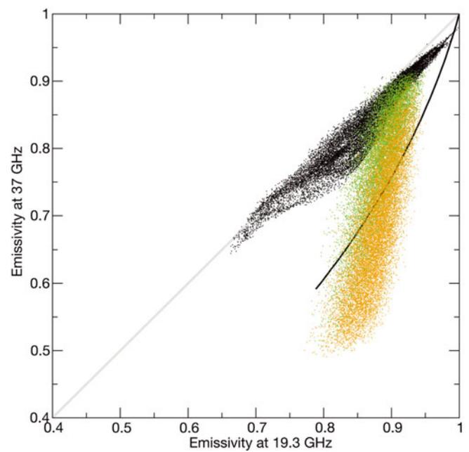
**Fig. 4.** Modeled emissivities at vertical polarization for snowpacks with a fixed snow grain radius (0.7 mm) and 15 layers with random variations of snow density in the first 10 m. Snowpacks were classified in two categories depending on the increase (orange color) or decrease (green color) of the density trend with depth. The curve represents the emissivity of homogeneous snowpacks (DMRT-ML calculation, grain radius of 0.1–1 mm; Fig. 3). Black dots are the observed emissivities.
