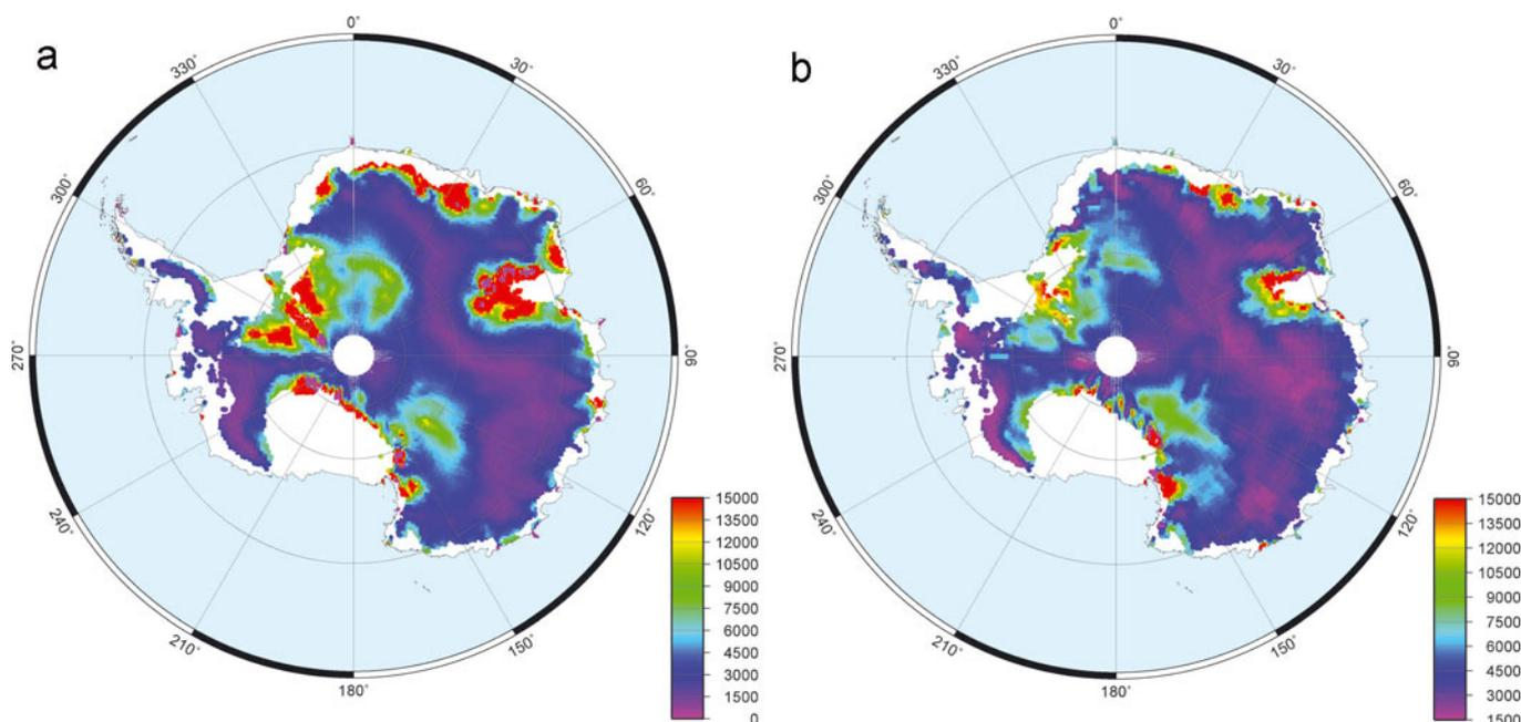
**Fig. 8.** Map of the gradient of grain size,  $Q^{\text{clim}}$  ( $\mu\text{m}^2 \text{m}^{-1}$ ), deduced from metamorphism theory (Equation (5)) using climatic data from (a) the MAR model and (b) the LMDZ4 model.
