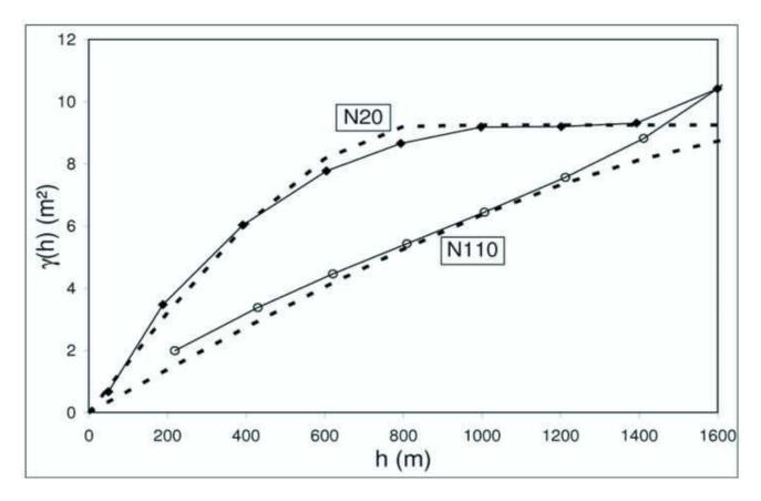
Fig. 6 Experimental semivariogram of reservoir bottom elevations direction N20 (smallest variance) and N110 (largest variance) of Akdarya reservoir.
