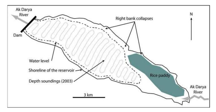
Fig. 4 Data measurements with bathymetric system CEEDUCER and current conditions of Akdarya reservoir in 2003
