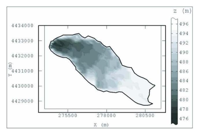
Fig. 7 Bathymetric map of Akdarya reservoir by kriging interpolation method
