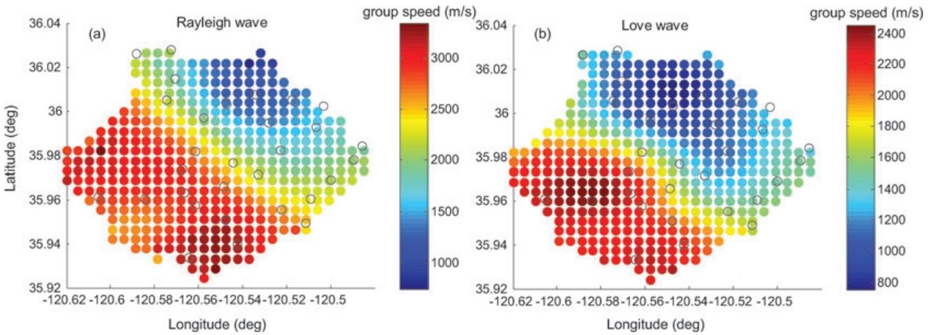
**Figure 6.** Group-speed velocity maps for (a) the Rayleigh wave and (b) the Love wave in the (0.1–0.2 Hz) frequency bandwidth for traveltime information accumulated over 15 consecutive days (Julian days 16–30) and extracted from the optimal noise-correlation tensor  $[\hat{C}_{AmBm}(t)]_{ij}$ . Black circles correspond to station locations.
