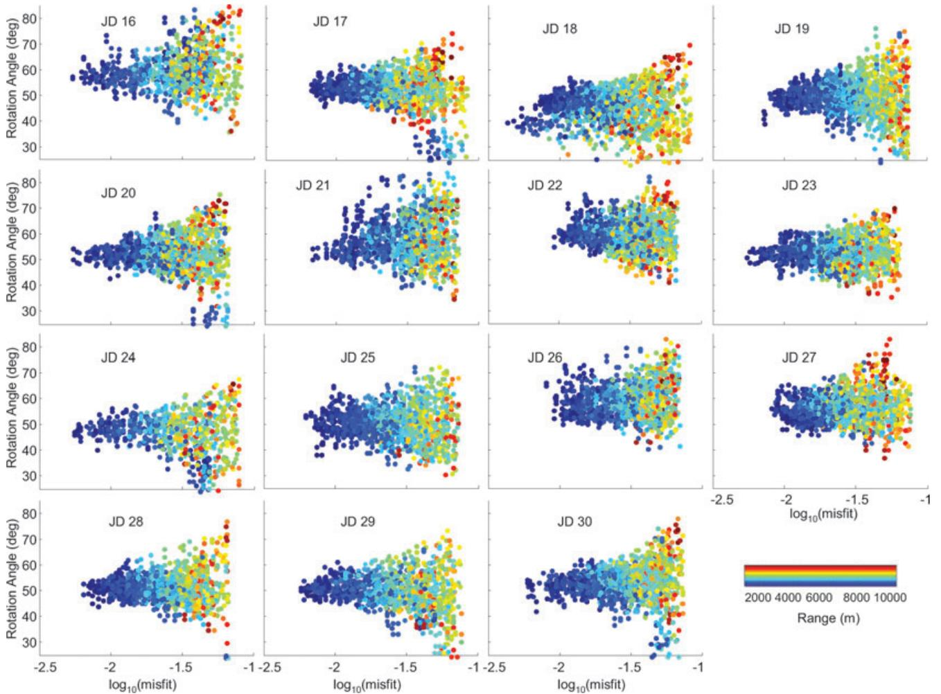
**Figure 5.** Day-by-day representation of the optimal azimuthal rotation angle  $\psi_m$  versus the optimal rotation misfit for each station pair. Misfit values were calculated as the total energy on components ZT, TZ, RT and TR of the optimal noise-correlation tensor  $[\hat{C}_{AmBm}(t)]_{ij}$  normalized according to the total energy of all of the components. The colour scale corresponds to the range between station pairs.
