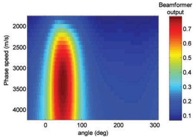
**Figure 2.** Angular-speed distribution of pre-processed incoming noise on the Parkfield network averaged over 1 d. Plane-wave beam-forming is summed incoherently over 100 frequencies from 0.1 to 0.2 Hz. The  $x$ -axis corresponds to noise directivity  $\theta_0$  (North is 0°, positive rotation is clockwise), the  $y$ -axis to speed  $c$ . Units are arbitrary.
