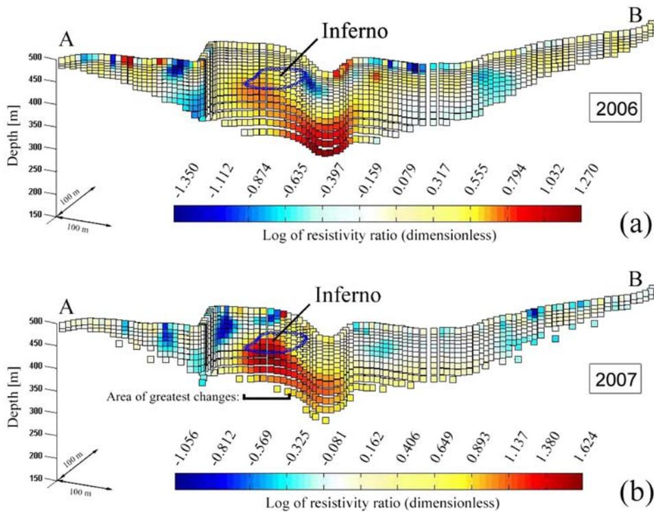
**Figure 3.** The distribution of the logarithm of resistivity ratio between overflow stage and recession stage (chosen as reference), performed in 2006 and 2007 along profile A–B shown in Figure 1; the blue circle represents the Inferno Lake location.
