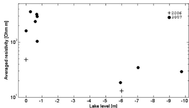
**Figure 5.** Averaged resistivity versus lake level in 2006 and 2007 computed on an area indicated on Figure 3 where the greatest changes are observed in 2007. The greatest changes in 2006 are located just outside this area (see Figure 3), which explains the lower resistivity values for 2006.
