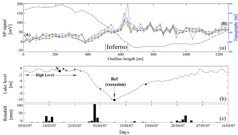
**Figure 2.** Results for self-potential survey. (a) Self-potential measurements along profile A–B in Figure 1, taken at different stages of Inferno cycle (see the corresponding colors above in Figure 2b). (b) Time at which the surveys have been performed over a whole cycle. “Ref” stands for the state chosen as reference to compute the resistivity ratio in Figure 3, and “N” stands for the high lake level state. (c) Rainfall data.
