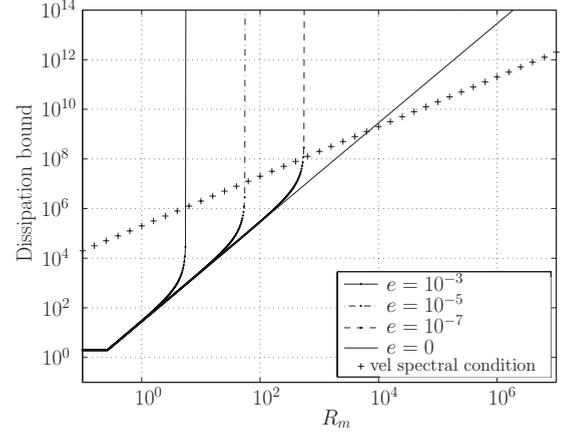
FIG. 2. Bound on dissipation obtained from Eq. (17) for the velocity spectral condition (“plus” signs) and from Eq. (28) for the magnetic spectral condition, for different wall conductances  $e = 10^{-3}$ ,  $10^{-5}$ ,  $10^{-7}$  and 0 plotted here for  $P_m = 10^{-5}$ .
