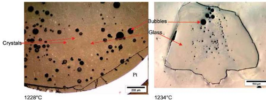
Figure 13. Glass balls quenched at 1228 and 1234 °C for composition C1 with sealed capsule.
