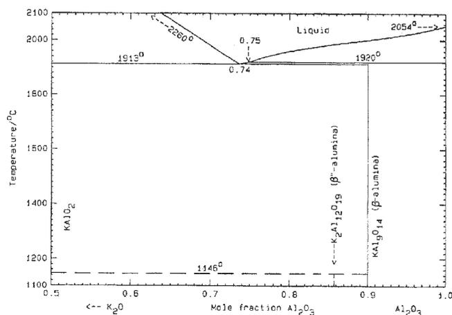
**Figure 1.** Binary diagram K<sub>2</sub>O–Al<sub>2</sub>O<sub>3</sub> [4].**Table 2. Liquidus Temperatures for C1 and C2 with and without Na<sub>2</sub>O and K<sub>2</sub>O**
