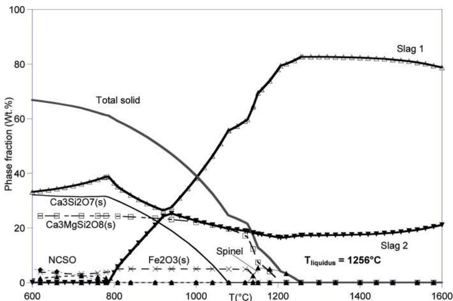
Figure 6. Weight percent of the phases formed as a function of the temperature for C2 with Na<sub>2</sub>O and K<sub>2</sub>O.
