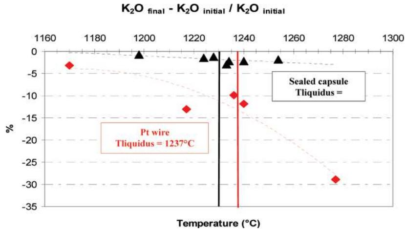
Figure 12. Evolution of K<sub>2</sub>O with and without capsule as a function of the temperature in comparison with the initial composition C1.
