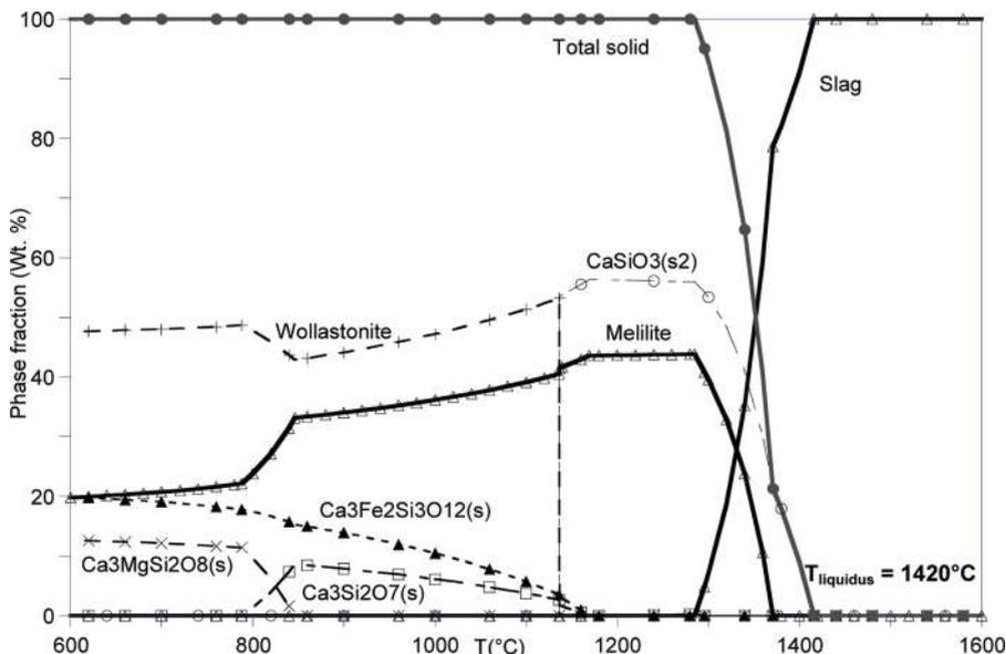
Figure 5. Weight percent of the phases formed as a function of the temperature for C2 without Na<sub>2</sub>O and K<sub>2</sub>O.
