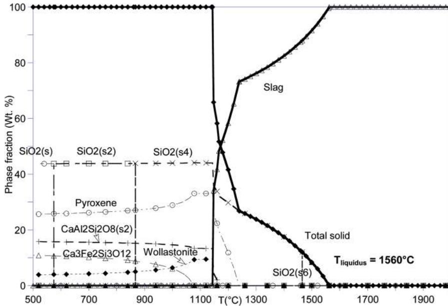
Figure 3. Weight percent of the phases formed as a function of the temperature for C1 without  $\text{Na}_2\text{O}$  and  $\text{K}_2\text{O}$ .
