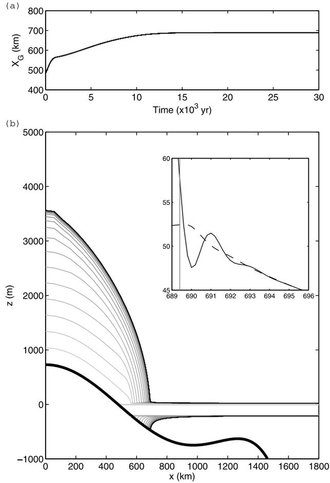
**Figure 2.** (a) Evolution of  $x_G$  over time for the first step of simulation HYST. (b) Surface profiles plotted every 1000 years. The steady state surface is plotted in black. The inset shows an enlargement of the upper surface (solid line) and is compared to the profile obtained for the floating surface (dashed line), whereas the vertical gray line marks the position of  $x_G$ .
