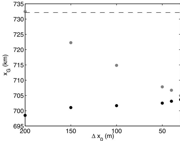
**Figure 6.** Evolution of the steady grounding line position as a function of the horizontal mesh extension  $\Delta x_0$ . Black circles (gray circles) represent results obtained for simulations starting from the steady state obtained after HYST step 2 (HYST step 12). Dashed line depicts results obtained by BL theory (Schoof, personal communication, 2008).
