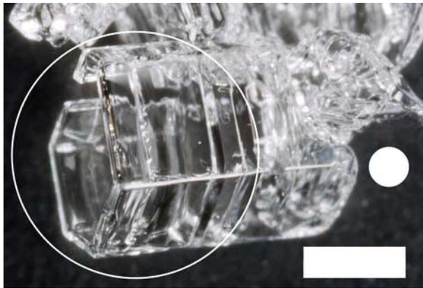
**Figure 1.** Photomicrograph of a depth hoar crystal with  $SSA = 167 \text{ cm}^2 \text{ g}^{-1}$  (see text). The scale bar is 1 mm. The white disc represents an ice sphere of radius  $r_e = 196 \mu\text{m}$  that has a  $SSA$  of  $167 \text{ cm}^2 \text{ g}^{-1}$ . The white circle, of radius 1.20 mm, has the same cross-sectional area as the depth hoar crystal. The  $SSA$  of ice spheres of that radius is  $27 \text{ cm}^2 \text{ g}^{-1}$ .
