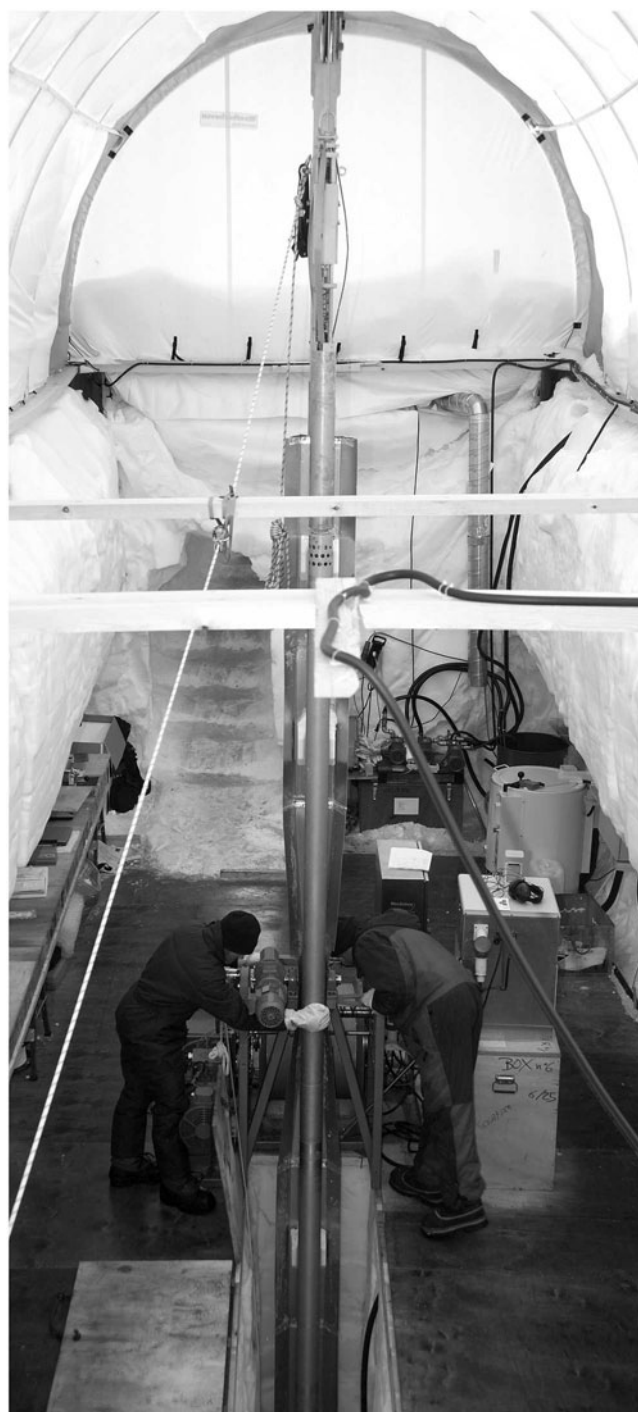
Fig. 9. The covered drilling pit, with deep ice-core drill system.
