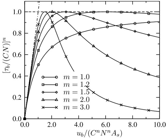
**Figure 8.** Proposed phenomenological friction law for different values of the parameter exponent  $q$ . Using these axes definition, the shape of the curves is not modified by a change in the two other parameters  $C$  and  $A_s$ . Same definition applies for dashed and dash-dotted lines as given in Figure 2.
