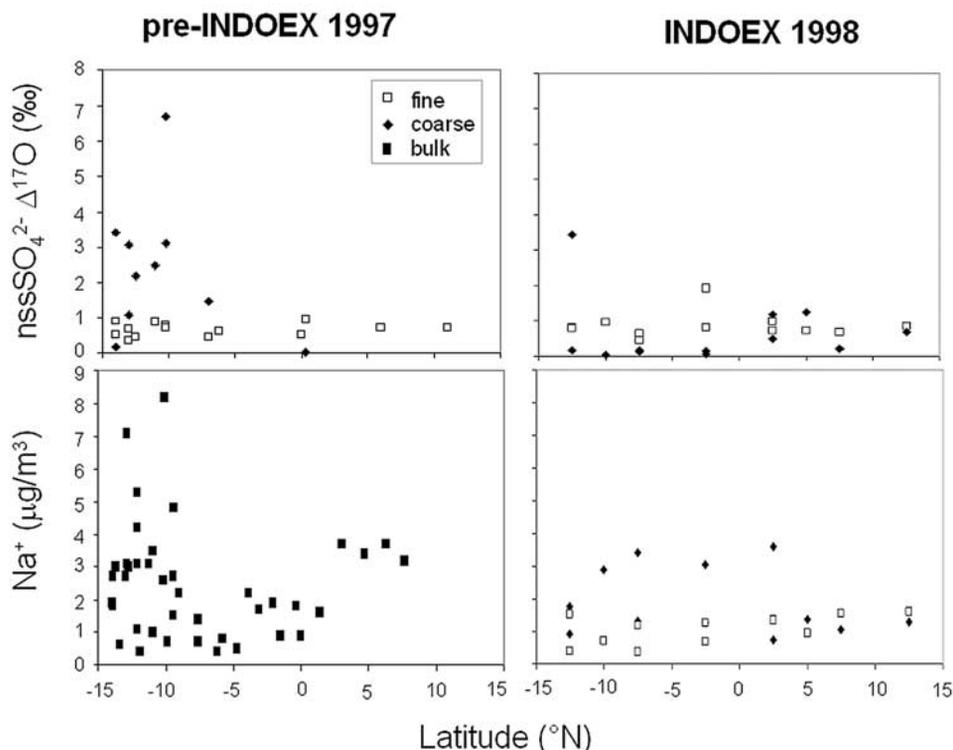
**Figure 3.** Measurements of (top) non-sea-salt sulfate ( $\text{nssSO}_4^{2-}$ )  $\Delta^{17}\text{O}$  and (bottom)  $\text{Na}^+$  concentrations for pre-INDOEX 1997 and INDOEX 1998. The data are segregated as fine ( $<1 \mu\text{m}$  diameter, open squares) and coarse ( $>1 \mu\text{m}$  diameter, solid diamonds) aerosols for all but  $\text{Na}^+$  for the 1997 pre-INDOEX cruise. Solid squares are bulk aerosol measurements from D. L. Savoie (personal communication, 2004).
