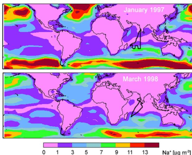
**Figure 2.** Simulated monthly mean sea-salt  $\text{Na}^+$  concentrations ( $\mu\text{g m}^{-3}$ ) in January 1997 and March 1998 averaged over the 0–100 m altitude column. Cruise tracks for the 1997 pre-Indian Ocean Experiment (INDOEX) cruise and the 1998 INDOEX cruise are shown as thick lines.
