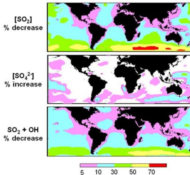
**Figure 7.** Effect of sea-salt chemistry on simulated yearly mean  $\text{SO}_2$  concentrations, sulfate concentrations, and the rate of gas phase sulfate formation ( $\text{SO}_2 + \text{OH}$ ) in the marine boundary layer at 0–100 m altitude.
