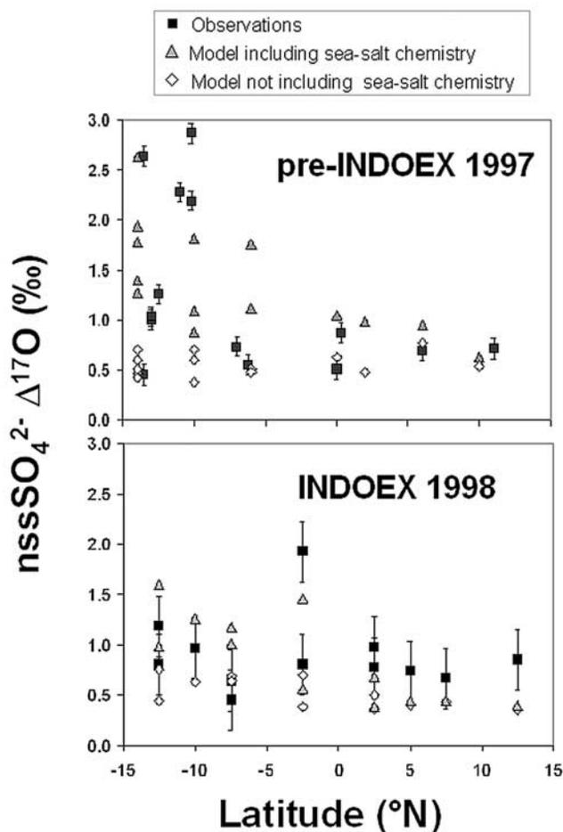
**Figure 5.** Bulk  $\text{nssSO}_4^{2-} \Delta^{17}\text{O}$  plotted as a function of latitude for the (top) 1997 pre-INDOEX and (bottom) 1998 INDOEX cruises. Observations (squares) are compared to model simulations including (triangles) and not including (diamonds) the production of sulfate in sea-salt aerosols.
