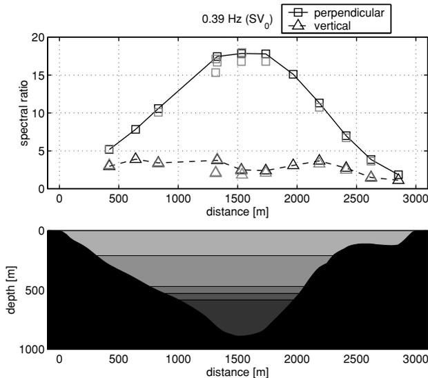
**Figure 22.** Average spectral ratios of 2003 experiment (first and second configuration) for vertical and perpendicular component as a function of distance along the profile at frequency 0.39 Hz, interpreted as mode  $SV_0$ . Values for the first configuration are connected with lines and plotted black.
