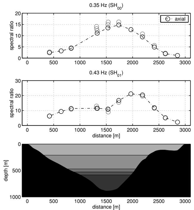
**Figure 23.** Average spectral ratios of 2003 experiment (first and second configuration) for the axial component as a function of distance along the profile at frequencies 0.35 (top) and 0.43 (bottom) Hz, interpreted as modes  $SH_{00}$  and  $SH_{01}$  respectively. Values for the first configuration are connected with lines and plotted black.
