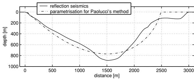
**Figure 6.** Sediment-bedrock interface of the Rhône valley at the Vétroz site derived from reflection seismics and described by eq. (4) with  $a = 1120$  m,  $h = 770$  m and  $\zeta = 0.20$  (modified from Schmid 2000).
