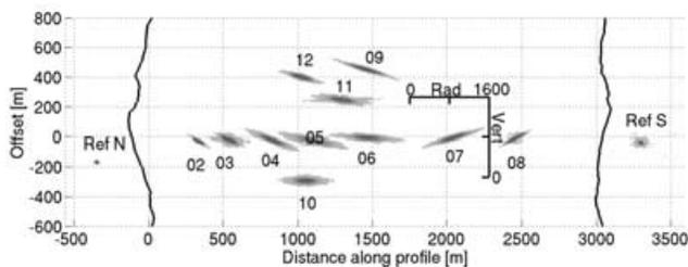
**Figure 29.** Particle motion plot of perpendicular vs. vertical component obtained from traces bandpass filtered between 0.32 and 0.38 Hz with noise recorded during the 2002 experiment. Areas passed multiple times are shaded dark.
