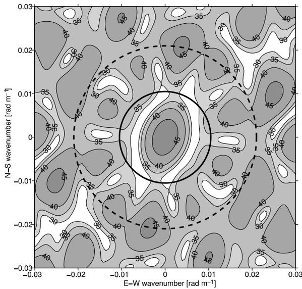
**Figure 9.** Beam pattern of array used for  $f-k$  analysis of 2002 experiment. Contour intervals are indicating the array response in dB. The first aliasing peaks are located on the dashed circle and the wavenumber domain that can be analysed with this configuration is within the solid circle.
