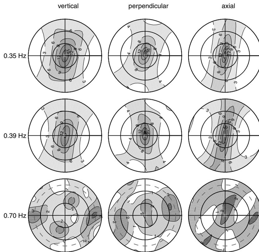
**Figure 30.**  $f$ - $k$  spectra as a function of slowness and azimuth for different frequencies and components. Azimuth is 0 on top (North). Slowness starts at zero (middle) and reaches  $3 \text{ s km}^{-1}$  at the outermost ring; concentric grid-lines denote slowness intervals of  $1 \text{ s km}^{-1}$ . Contour intervals are given in dB. The grey dashed line at  $0.70 \text{ Hz}$  shows the Nyquist slowness.
