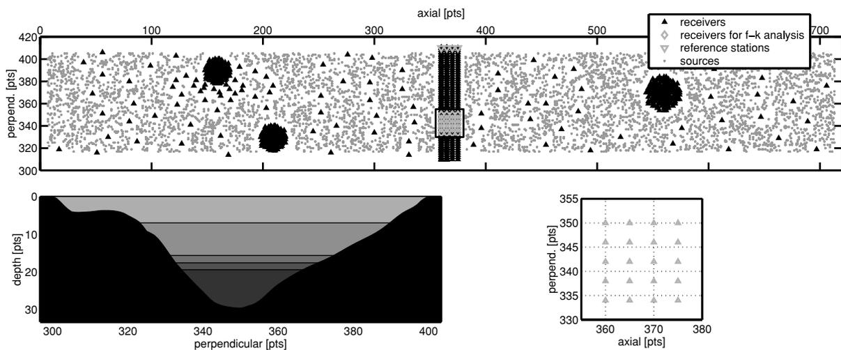
**Figure 10.** *Top:* Source and receiver distribution used for numerical simulation of microtremor. Distances are in grid points, the grid spacing is 30 m. *Bottom left:* Cross-section of velocity model. *Bottom right:* Enlarged section showing the array used for  $f-k$  analysis.
