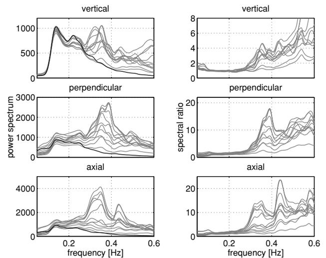
**Figure 20.** Average power spectra (left) and average site-to reference spectral ratios (right) calculated from ambient noise recorded during the 2003 Vétroz experiment (first configuration). Power spectra of reference receivers located on bedrock are plotted black. The reference station is ‘Ref’ shown in Fig. 7.
