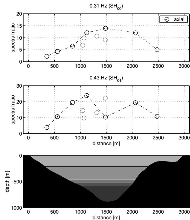
**Figure 19.** Average spectral ratios of 2002 experiment for axial component as a function of distance along the profile at 0.31 (top) and 0.43 (bottom) Hz. Points located on the profile are connected with lines.
