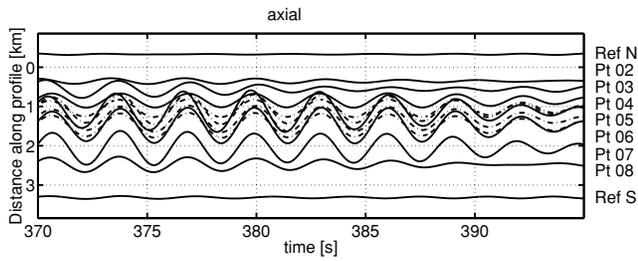
**Figure 24.** Time window of ambient noise recorded on the axial components during the 2002 experiment bandpass filtered around  $SH_{00}$  between 0.28 and 0.34 Hz. Seismograms of points outside the profile are printed with dashed lines.
