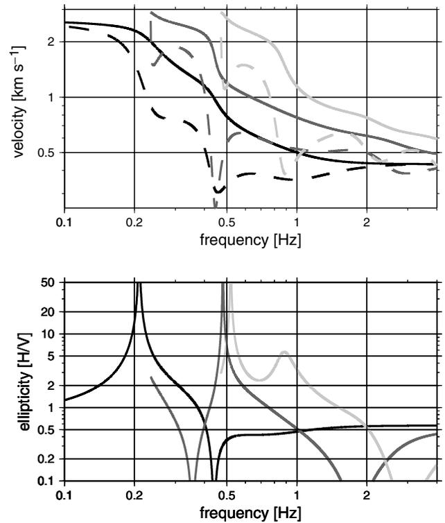
**Figure 2.** 1-D dispersion analysis of velocity model given in Table 1 *Top:* Phase (solid) and group velocities (dashed) for fundamental (black), first (dark grey) and second (light grey) higher mode Rayleigh waves. *Bottom:* Particle-motion horizontal/vertical ratios for the same modes, same model. (These values were computed using software from Hermann 2002).
