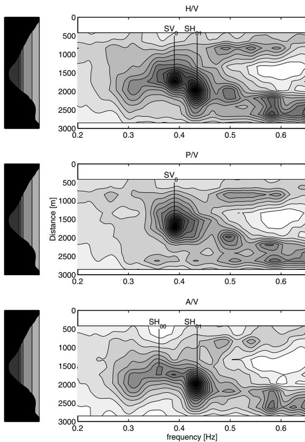
**Figure 31.** Horizontal-to-vertical spectral ratios as a function of distance along the profile and frequency. Top: horizontal/vertical, centre: perpendicular/vertical, bottom: axial/vertical. (2003 experiment, first configuration).
