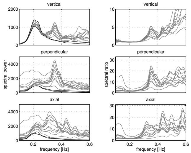
**Figure 17.** Average power spectra (left) and average spectral ratios (from the reference station in the North, right) calculated from ambient noise recorded during the 2002 Vétroz experiment. Power spectra of reference receivers located on bedrock are plotted black.
