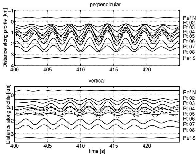
**Figure 25.** Time window of perpendicular (top) and vertical (bottom) components bandpass filtered around  $SV_0$  between 0.32 and 0.38 Hz. Seismograms of points outside the profile are printed with dashed lines. (2002 experiment)
