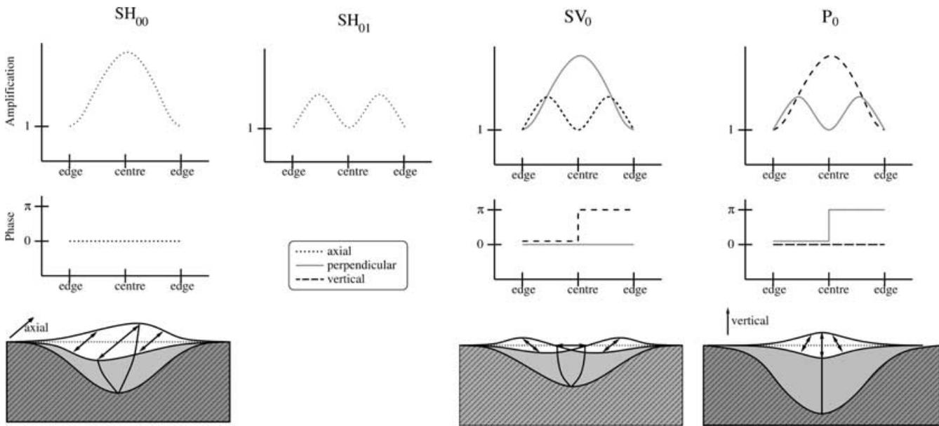
**Figure 4.** Amplification, phase and particle motion of the three fundamental modes of a sine shaped valley for the corresponding critical shape ratio (modified from Bard & Bouchon 1985; Steimen *et al.* 2003) and amplification for the first higher mode  $SH_{01}$ .
