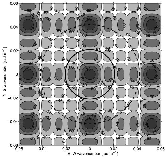
**Figure 15.** Beam pattern of array configuration for  $f-k$  analysis of synthetic microtremors. Contour intervals are indicating the array response in dB. The dashed circle indicates the wavenumber where the first aliasing peaks occur and the solid circle shows the Nyquist wavenumber.
