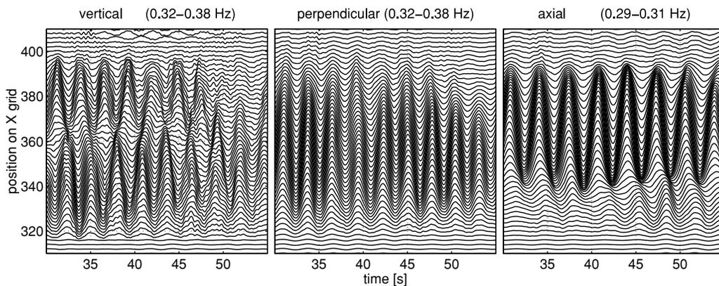
**Figure 14.** Bandpass filtered synthetic ambient noise records for all points on profile at axial grid position 370. The bandpass was applied at the  $SV_0$  (vertical, perpendicular) and  $SH_{00}$  (axial) fundamental mode frequency.
