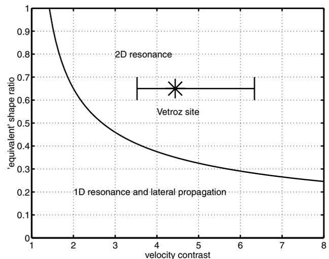
**Figure 5.** Critical shape ratio as a function of the velocity contrast for the  $SH$  case. The velocity contrasts obtained from the shear-wave velocities in Table 1 are indicated at the shape ratio of 0.65. The asterisk denotes the velocity contrast obtained with the traveltime-based shear-wave velocity average from eq. (1). (modified from Bard & Bouchon 1985).
