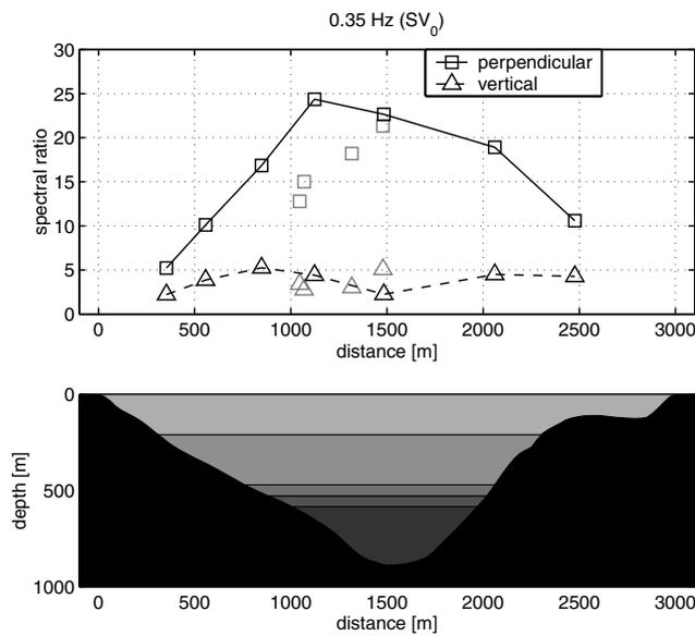
**Figure 18.** Average site-to-reference spectral ratios for ambient noise recorded in the 2002 experiment for vertical and perpendicular component as a function of distance along the profile (from North to South). Points located on the profile axis (Nr. 02-08 in Fig. 7) are connected with lines and plotted black, points located away from the axis are plotted grey. The reference station is ‘Ref N’ shown in Fig. 7.
