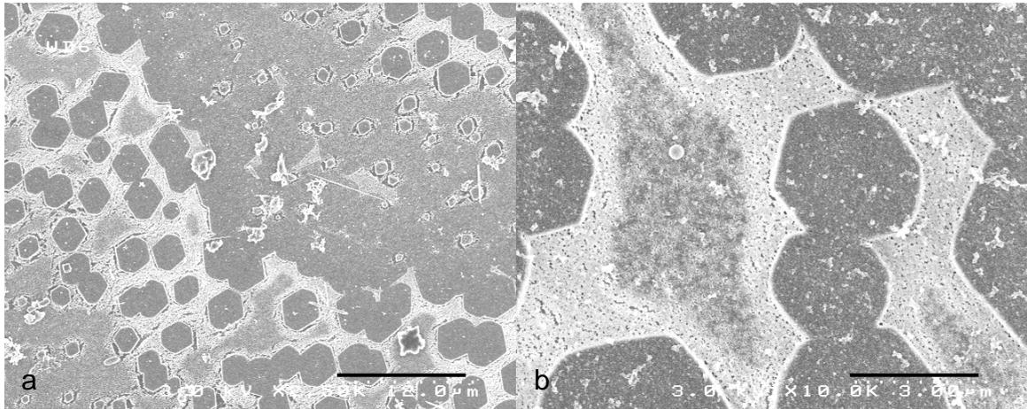
**Supp-Fig. 3.** Direct observation of nacre growing compartment surface on shell side at low magnification (a, scale bar = 12  $\mu\text{m}$ ) and higher magnification (b, scale bar = 3  $\mu\text{m}$ ). The samples were fixed in 70% ethanol and progressively dehydrated. Supp-Fig. 3 shows that the organic material keeps in place and appears white in SEM at low energy.
