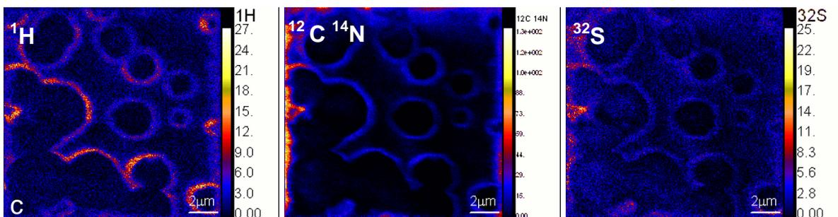
**Supp-Fig. 4.** Distribution of organics in growing nacre. The distribution of H, N, and S imaged with the NanoSIMS at the very surface of the growing nacre (row *a*), at depths of about 100 nm (row *b*) and at a depth of about 200 nm (row *c*). The organic-rich ring surrounding each tablet is clearly visible once overlying material has been removed (row *c*).
