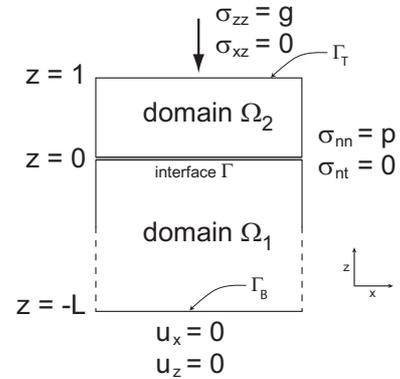
**Fig. 3.** Geometry of the system: two linear elastic solids with identical moduli are pushed into each other and separated by a thin confined water film at pressure  $p$ . The boundaries conditions used in Sections 3 and 4 are given.
