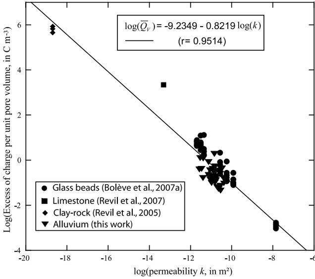
**Figure 1.** Dependence of the excess of charge per unit pore volume with the permeability at saturation of the porous materials. This data set includes various lithologies and salinities ( $6 \leq \text{pH} \leq 8.5$ ). The alluvium materials are from the Boise State University test site. They are composed of a mixture of sands and gravels.
