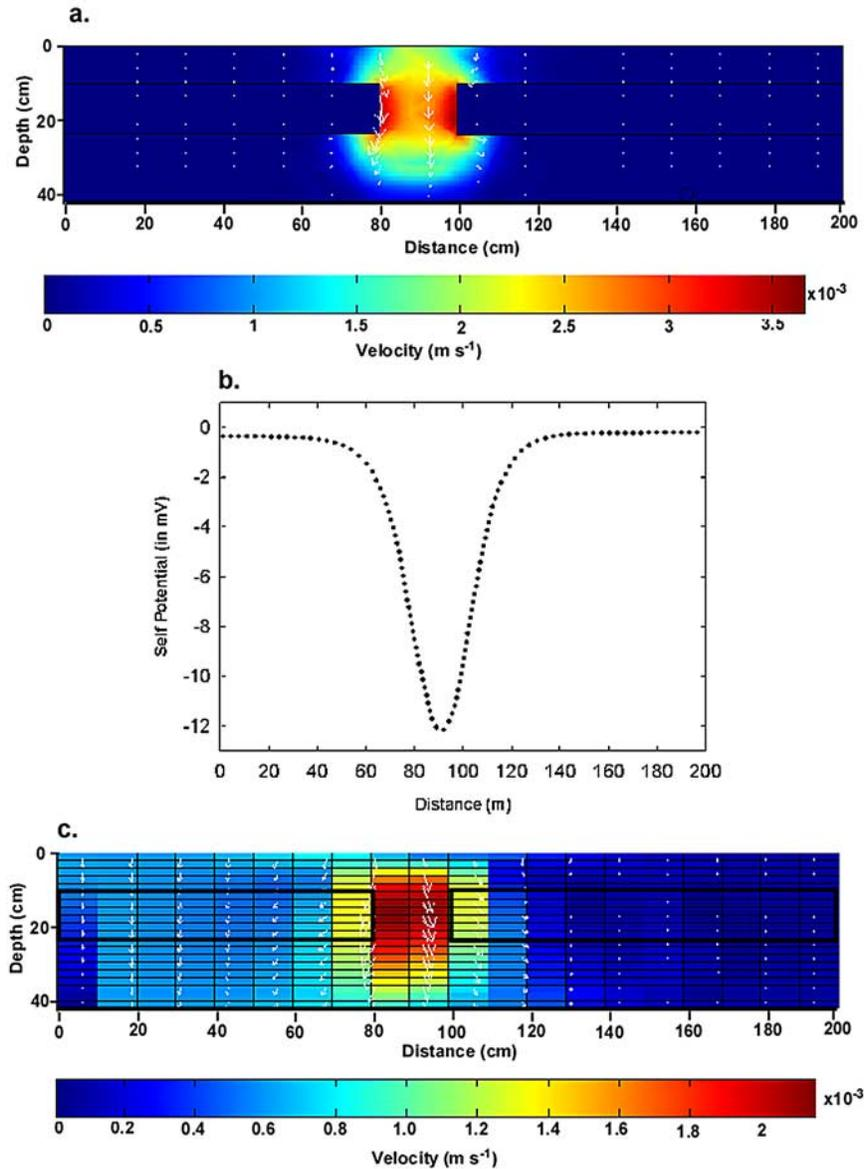
**Figure 3.** Synthetic case for a vertical 2D-infiltration problem. (a) True distribution of the Darcy velocity (in  $\text{m s}^{-1}$ ). (b) Distribution of the resulting self-potentials, which is sampled at the top surface of the system every meter. (c) Distribution of the reconstructed Darcy velocity ( $R^2 = 0.95$ ).
