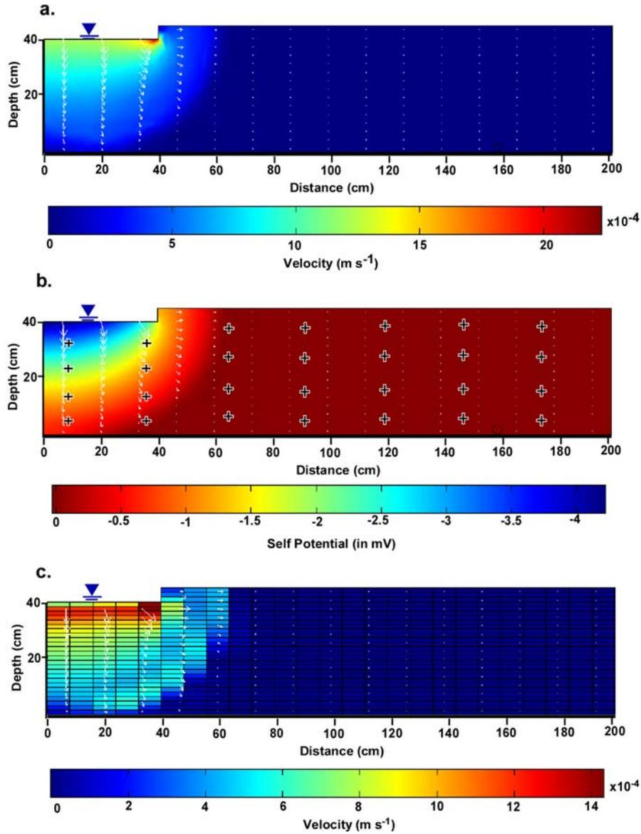
**Figure 2.** Synthetic case for the 2D-infiltration from a ditch. (a) The Darcy velocity is modeled from the Richard equation. (b) Distribution of the self-potential for the synthetic case. We assume that the «measurements» of the self-potentials are performed at the location with the symbols (+) are located. (c) Distribution of the reconstructed Darcy velocity ( $R^2 = 0.98$ ).
