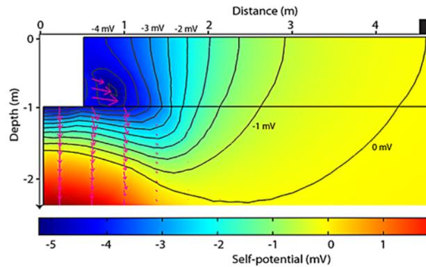
**Figure 5.** Simulated SP distribution and the Darcy velocity associated with the infiltration in the ditch of Roujan using all the hydraulic information available from in situ and petrophysical measurements [see Bolève *et al.*, 2007b].
