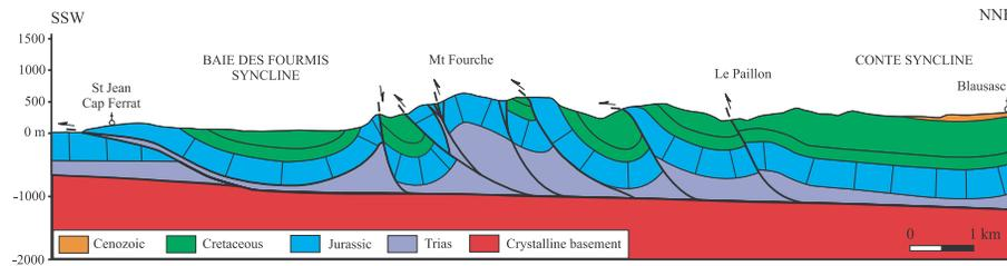
**Figure 4.** Geological cross-section from Blausasc to Cap-Ferrat (see Fig. 3 for location). The frontal part of the Nice arc corresponds to seven imbricate thrust-sheets made of sedimentary rocks from Triassic evaporites (décollement level) up to Cenozoic. At the frontal part of the belt, only the sedimentary cover appears to be thrust up, the crystalline basement is not involved by duplex structures.
