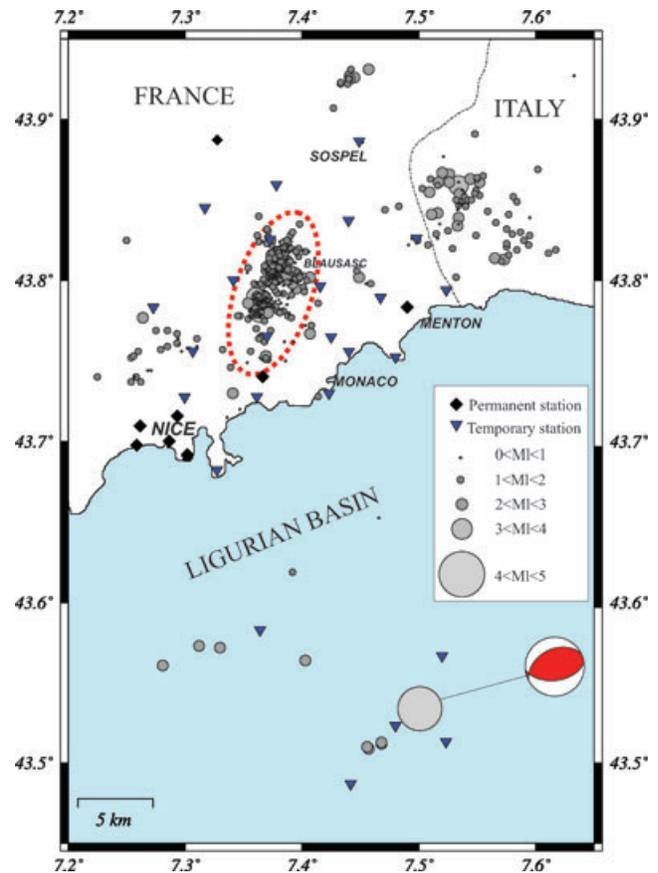
**Figure 6.** Localization and magnitude of the earthquakes recorded during the SALAM seismic experiment. The focal mechanism of the largest earthquake that occurred during the campaign (2001 February 25,  $Ml = 4.6$ ) has been computed using  $P$ -wave polarities on numerous stations. The red ellipse shows the location of the Blausasc sequence.
