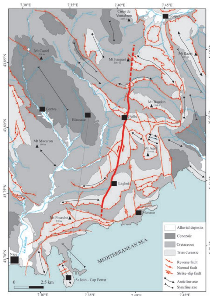
**Figure 3.** Tectonic map of the study area (frontal part of the Nice arc). The Peille-Laghet fault is in bold and the grey line from Blausasc to Saint Jean Cap-Ferrat corresponds to the geological cross-section of Fig. 4.
