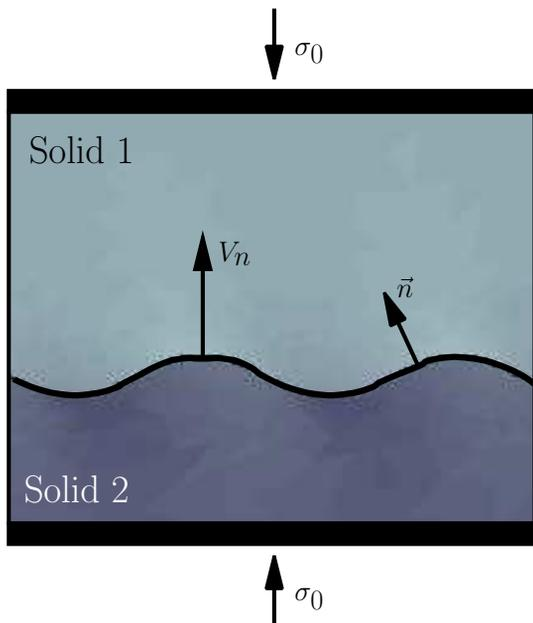
FIG. 1: (Color online) Basic setup of the model for a moving interface between two elastic solid phases, characterized by different Young's moduli ( $E_2 > E_1$ ) and Poisson's ratios  $\nu_1, \nu_2$ . The interface boundary propagates with a normal velocity  $V_n$ , when the solids are subjected to uniform far-field compressional stresses  $\sigma_0$  in the vertical direction.
