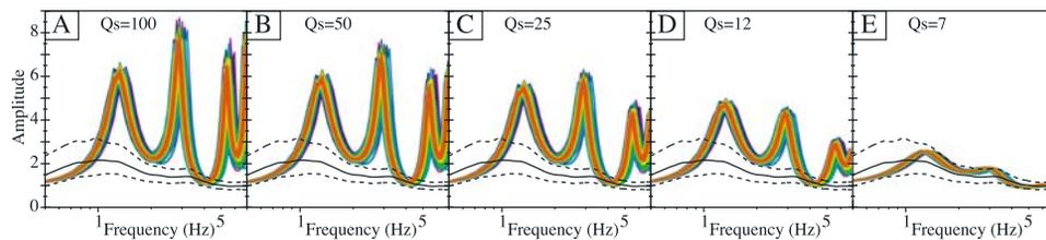
**Figure 4.** Averaged H/V (black solid line) and H/V standard deviation (black dashed lines), and transfer functions, from the selected models of the 134 m array, with  $Q_s = 100$  in the underlying half-space and  $Q_s$  in the upper layers of (a) 100, (b) 50, (c) 25, (d) 12, and (e) 7.
