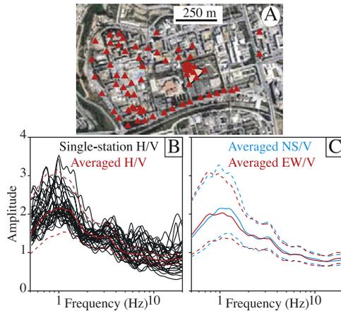
**Figure 1.** Single-station H/V results in the “Cité des 1200 Logements” of Boumerdes. (a) Location of H/V recordings (red triangles) and of microtremor arrays (pink triangle). (b) All single-station H/V curves (black lines) and the corresponding averaged H/V curve (red line) and standard deviations (red dashed lines). (c) Averaged N-S/V and E-W/V (solid lines) and standard deviations (dashed lines).
