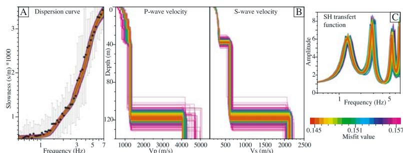
**Figure 3.** Two-layer analysis from the 134 m aperture array. Legend as for Figure 2. Two interfaces, at 37 m and 118 m, appear on both velocity profiles. The transfer functions exhibit two peaks at 1.3 Hz and 3 Hz.
