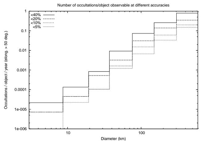
**Fig. 3.** Number of observable occultations per object during one year, as a function of the asteroid diameter, for a 20 cm telescope equipped with a cheap fast-readout camera. These statistics are valid for a single site and are computed for different values of the maximum relative uncertainty on size,  $\sigma_D$ , as indicated by the legend.
