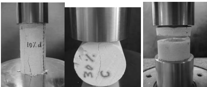
Figure 3: Mortar samples during compressive, tensile and adhesive tests respectively
