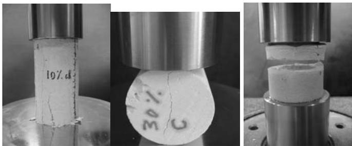
Figure 3: Mortar samples during compressive, tensile and adhesive tests respectively
