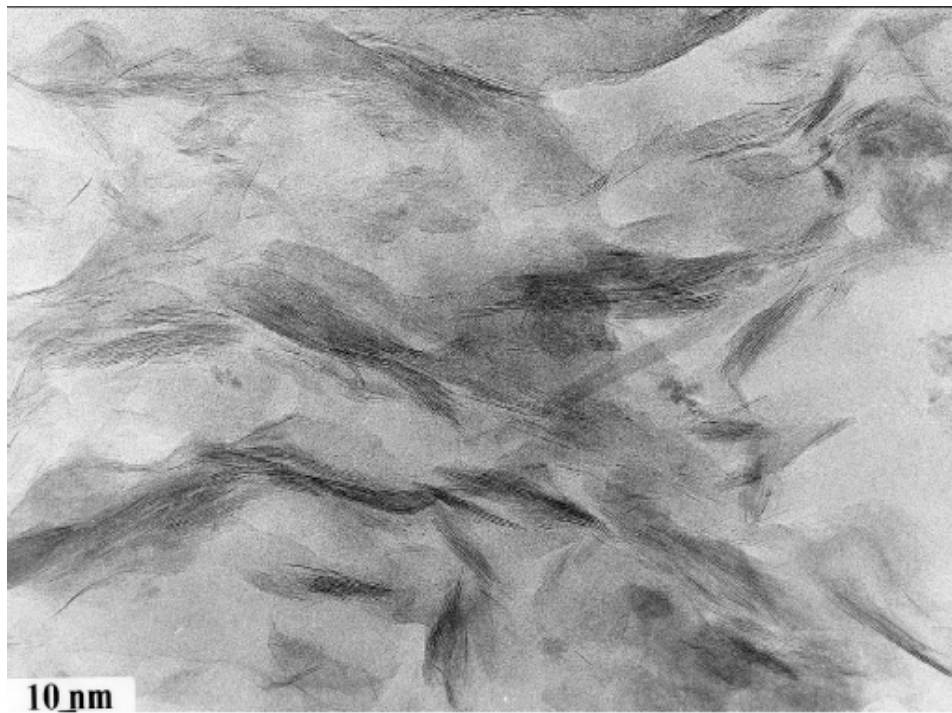
Figure 5. a) TEM image of Wyoming Mg-montmorillonite treated with 0.01M \text{Pb}(\text{NO}_3)_2 solution.
