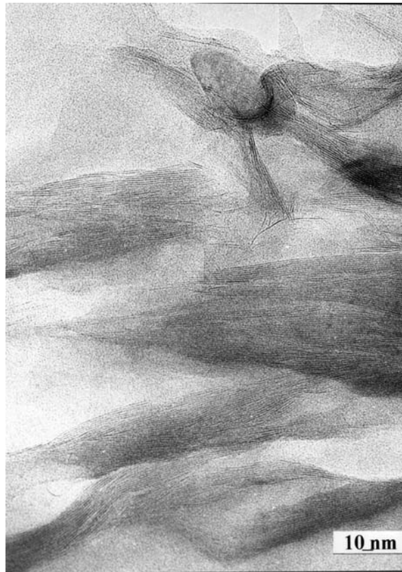
Figure 5. b) TEM image of Pprenjas bentonite treated with 0.01M \text{Pb}(\text{NO}_3)_2 solution with numerous little particles.
