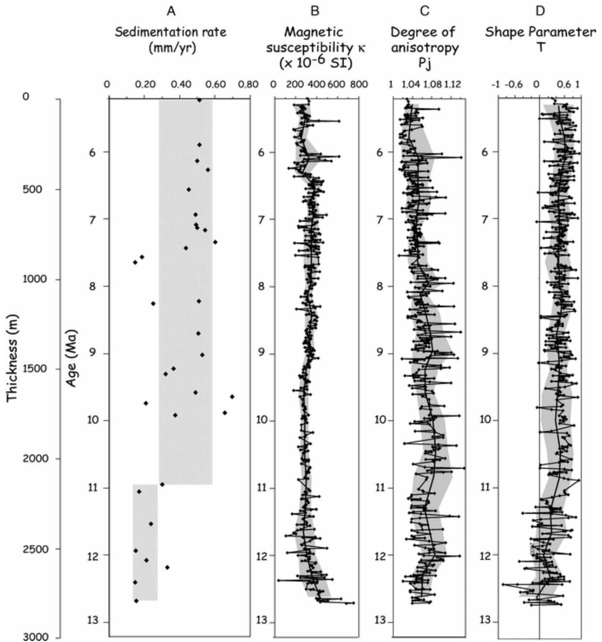
Figure 3. A: Plot of instantaneous sedimentation rate of data shown in [Figure 2D](#) (uncertainty envelope in gray). B: Magnetic susceptibility ( $\kappa$ ), (C) magnetic anisotropy, and (D) shape parameter  $T$  as function of depth and time for Yaha section
