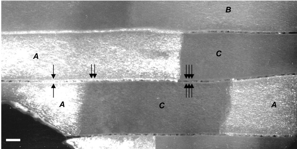
**Fig. 2.** Darkfield TEM image of nacre evidencing the crystalline structure of the organic matrix (bar is 100nm) . Organic matter is in contrast when under Bragg conditions whilst the mineral phase remains systematically extinguished.
