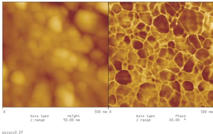
**Fig.3. AFM images of the polished surface of nacre tablets in tapping-mode (polished with tablets flat-on) : a) Topography of the surface (Height) b) Picture in Phase Contrast showing the foam-like structure of the intracrystalline organic matrix.**
