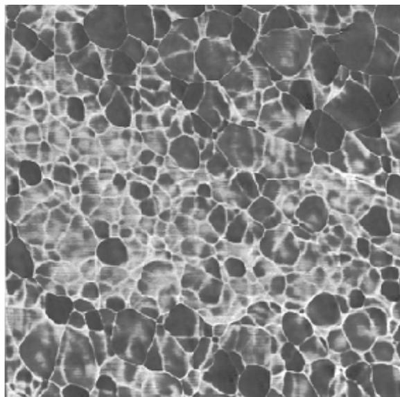
**Fig. 4. AFM picture in Phase Contrast ( $1 \times 1 \mu\text{m}^2$ ).**
