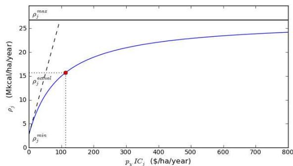
Figure 8: Yield in a land class as a function of chemical input consumption  $IC_j$ .  $\rho_j^{max}$ ,  $\rho_j^{actual}$  and  $\rho_j^{min}$  are the potential, actual and minimum yields of the land class  $j$ .  $p_\chi$  is the price index of chemical inputs.
