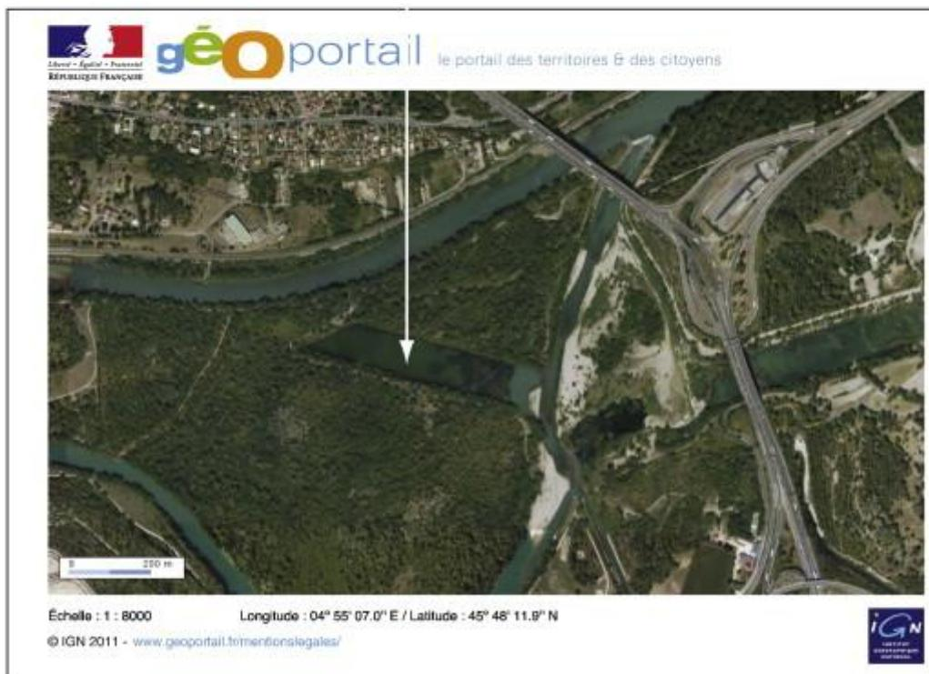
Fig. S-4. Map and aerial image of the coring site at Crépieux-la-Pape (CPX). The site is a former gravel quarry adjacent to the old channel of the Rhône River. It was formed at the beginning of the 1980s by dredging of alluvial deposits. The harbor-shaped feature left by quarrying is about 3 m deep at the center. Since quarrying ended in the early 1980s, flood deposits have formed a submerged levee that
